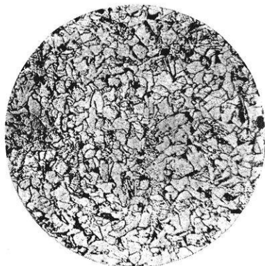
FIGS. 5 AND 6.— The Same Straight Carbon and Nickel Steels After Heating to 1,200° for One-half Hour and Slowly Cooling. 72 dia.
