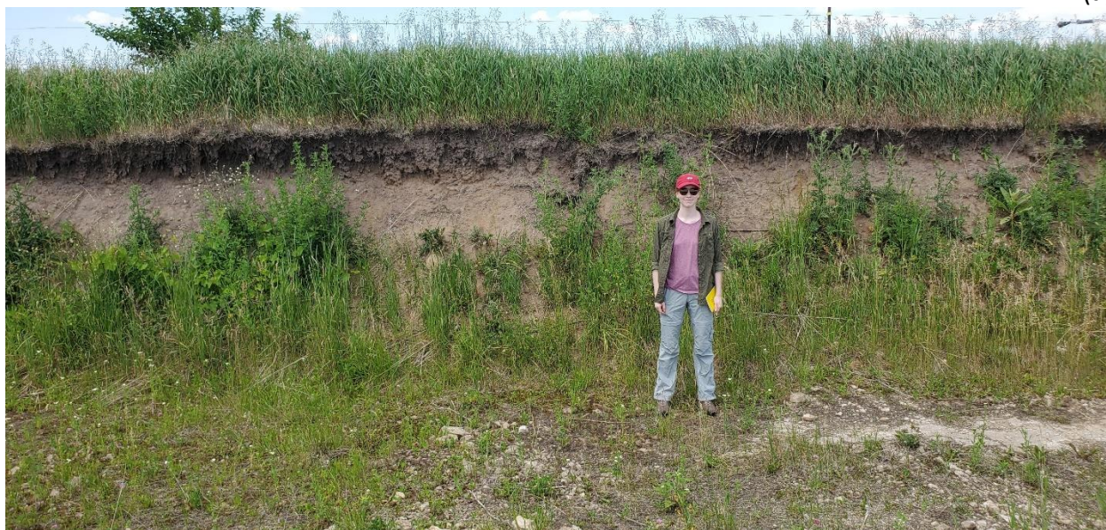
Figure B.36: Image of the South face of the testing (a) East end of the tested area (depth to bedrock \sim 0.4 m), and (b) West end of the tested (depth to bedrock \sim 1.8 m). The sediment depth increases from east to west. Ms. Katherine Swager served as the scale for the photographs.
