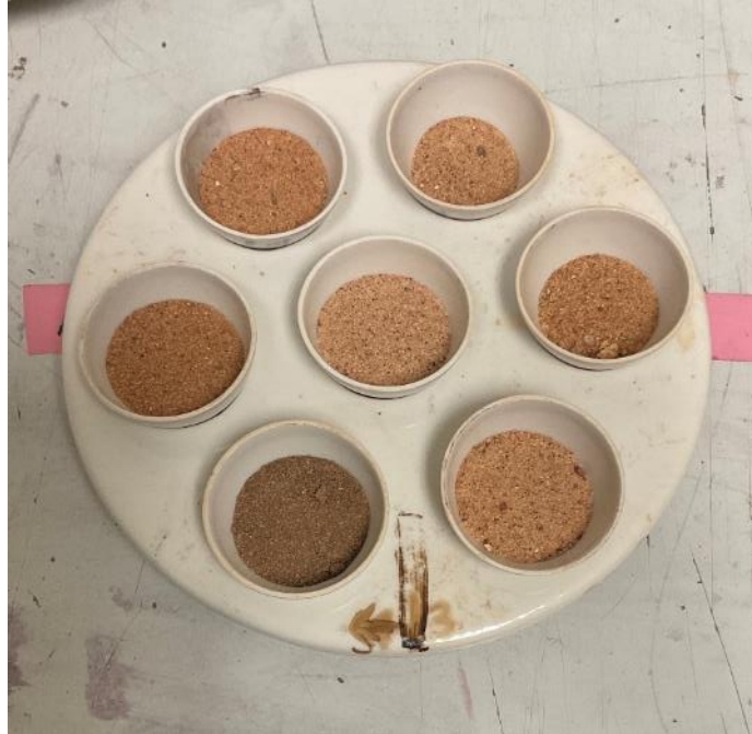
Figure A.10: Representative soil sample from 10-cm interval prepared for LOI testing.
