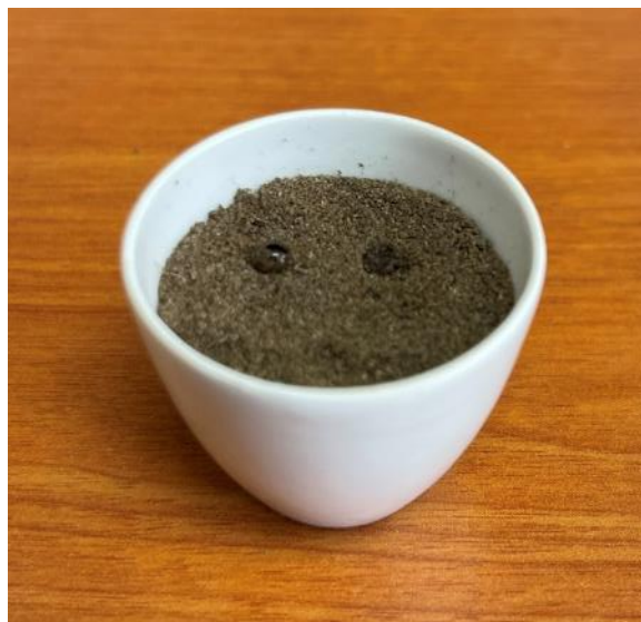
Figure A.22: Water droplet immediately after being placed onto the soil showing hydrophobic characteristics before being absorbed (left) next to a droplet already absorbed into the soil (right). This sample is from outside the infiltration testing area of the first 10 cm.
