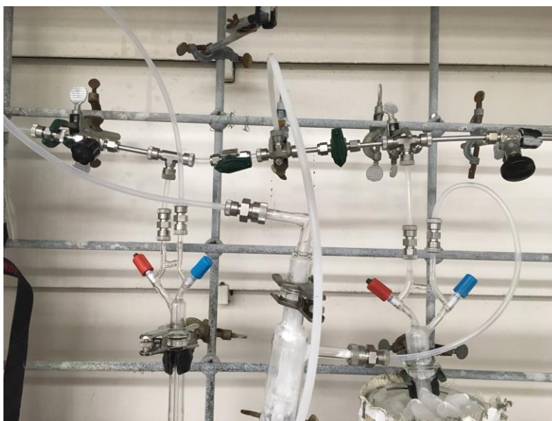
Figure 3. Photo taken of the \text{N}_2\text{O}_5 synthesis apparatus.
