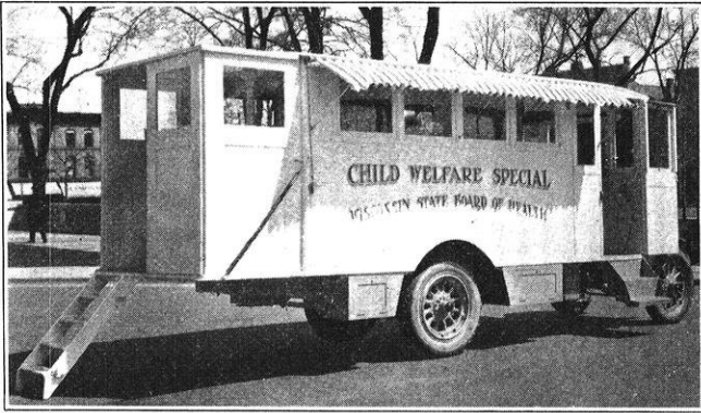
FIG. 1. THE CHILD WELFARE CAR UNLIMBERED FOR ACTION. The car is fully equipped with a hot water heating plant, lavatory and running water, and electric lights.
