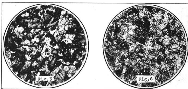
FIG. 5. .3% CARBON STEEL HELD 4 HOURS AT 900 C AND SLOWLY COOLED. X100
