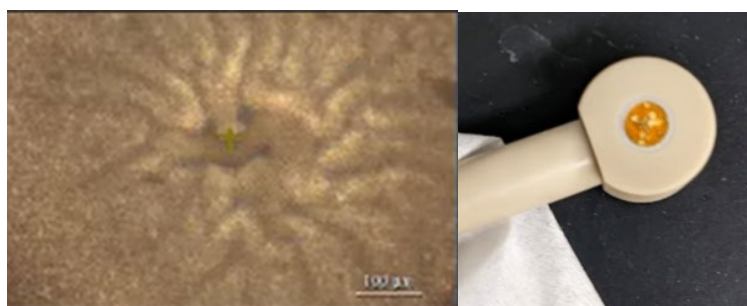
Figure 4.11 Picture of the electrode surface when a potential is stepped to -2.7 V vs. Ag/Ag + (left) showing the formation of solid precipitate that, when exposed to ambient humidity, forms an orange film (right).
