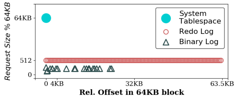
Figure 2.9: Write profile of MariaDB/InnoDB logs. The logs are contained in three files: (1) the System Tablespace file contains the undo log, doublewrite buffer, and the change buffer, (2) the Redo Log, and (3) the Binary Log for database replication. Read requests to these files follow a similar pattern. Write requests to the system tablespace file are multiples of 64KB (stripe size for SSD-S) aligning with internal stripes, and don't violate any rules. The write requests to the redo log are of size 512B (aligned with 512B boundaries), and violate Rules 1 & 3. The binary log on the other hand contains small write requests of varying sizes, which violate Rules 1, 3, and 5.
