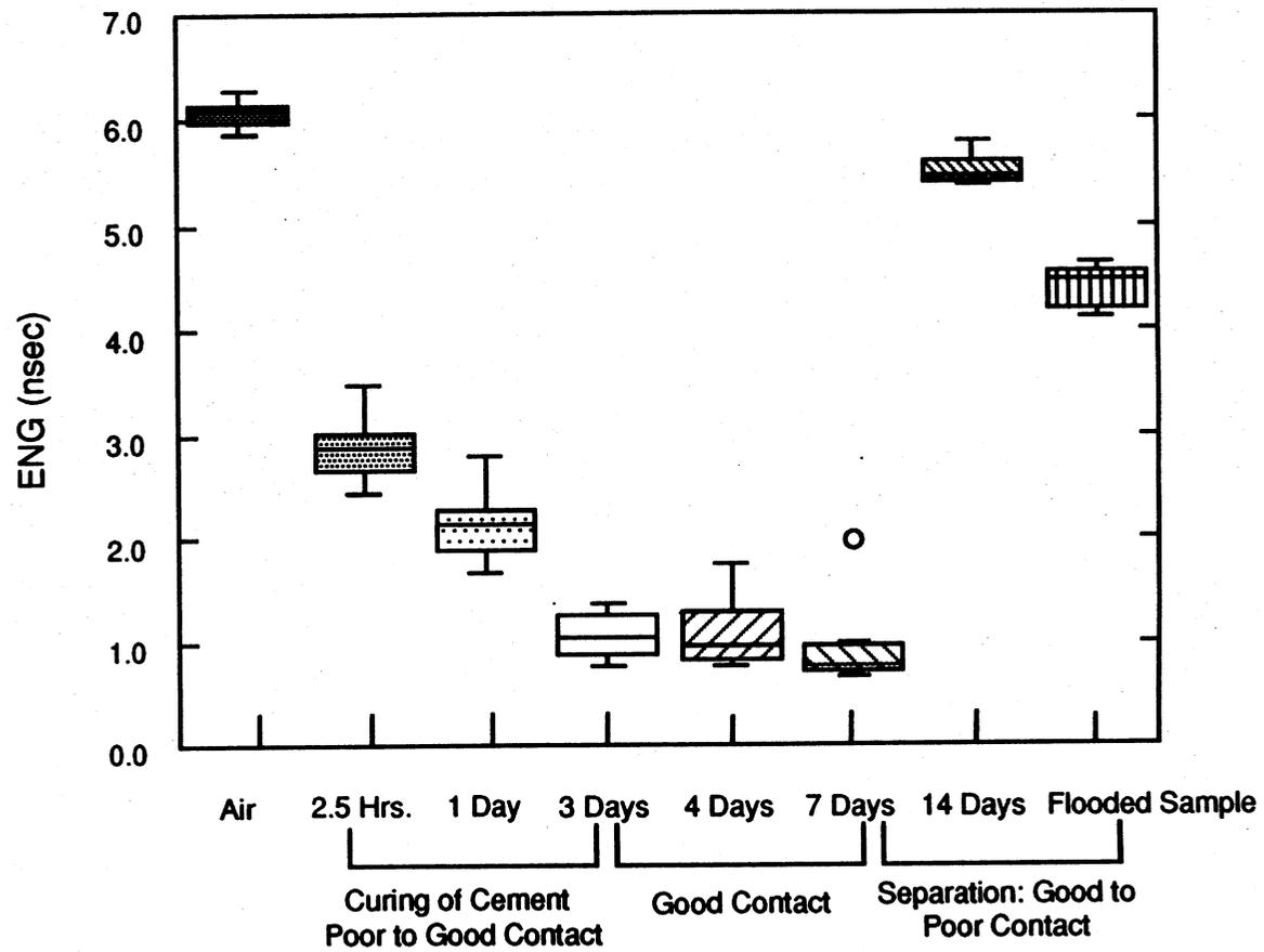
Fig. 3.9. ENG from Neat-Cement Specimen vs. Testing Time or Condition
