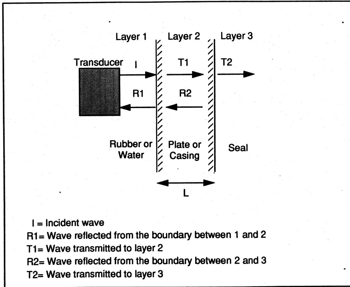
Fig. 3.2. Three Layered System Used in the Tests
