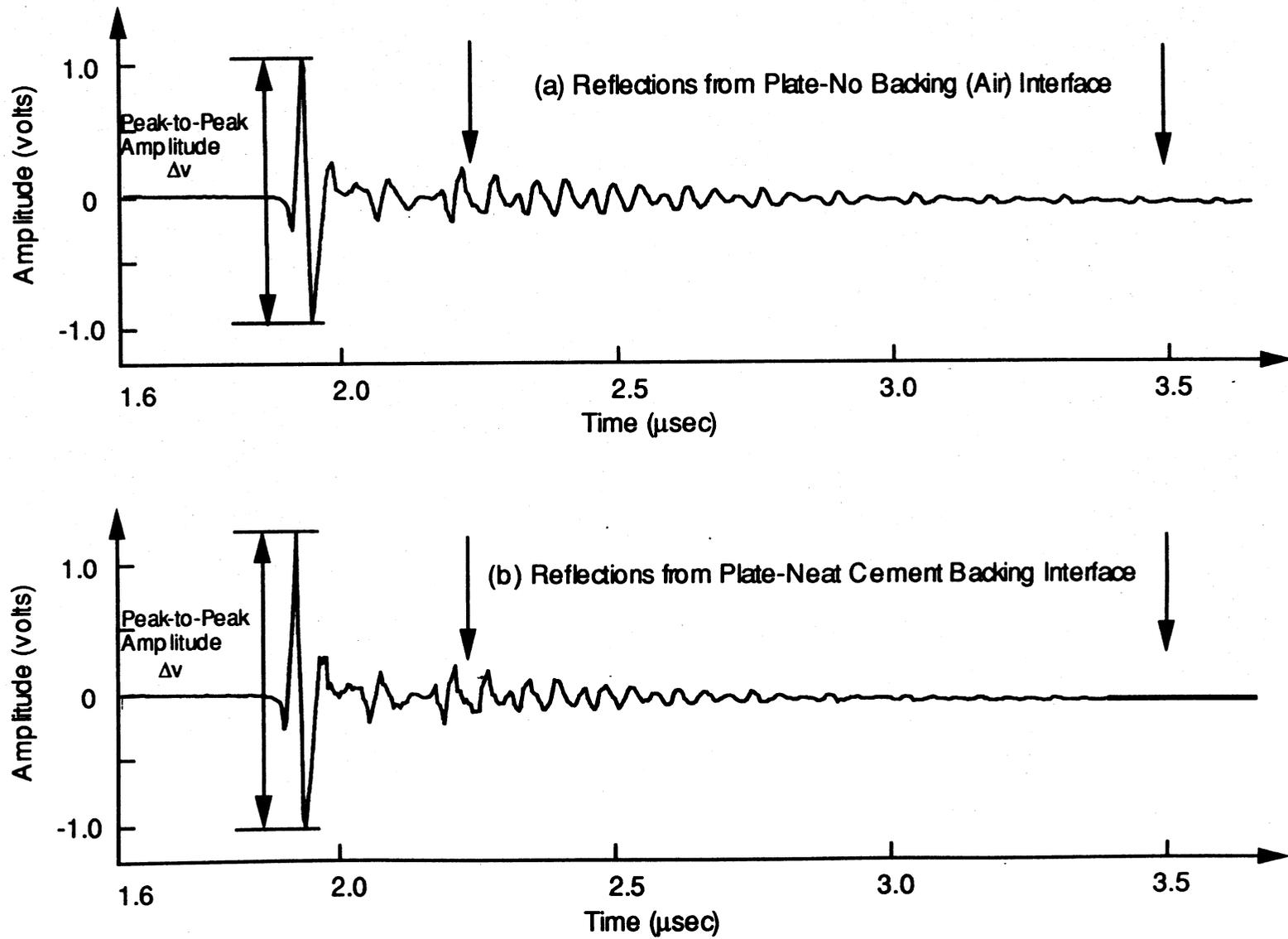
Fig. 3.6. Two Typical Waveforms Obtained in the Tests: No Backing and Neat Cement Backing
