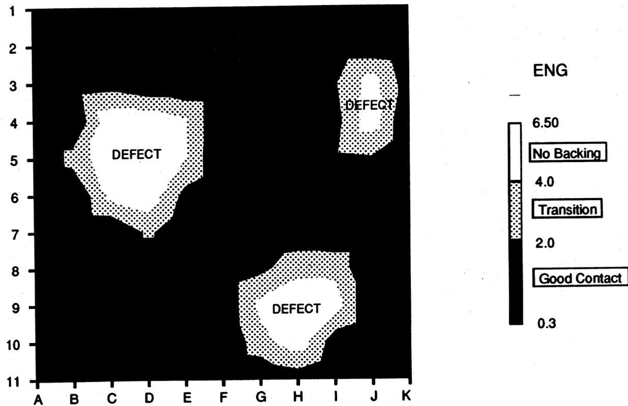
Fig. 3.13. Neat-Cement Specimen with Multiple Defects
