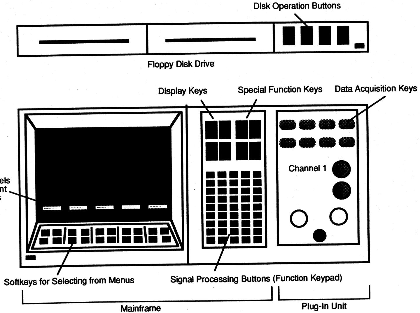
Fig.3.4. Waveform Analyzer
