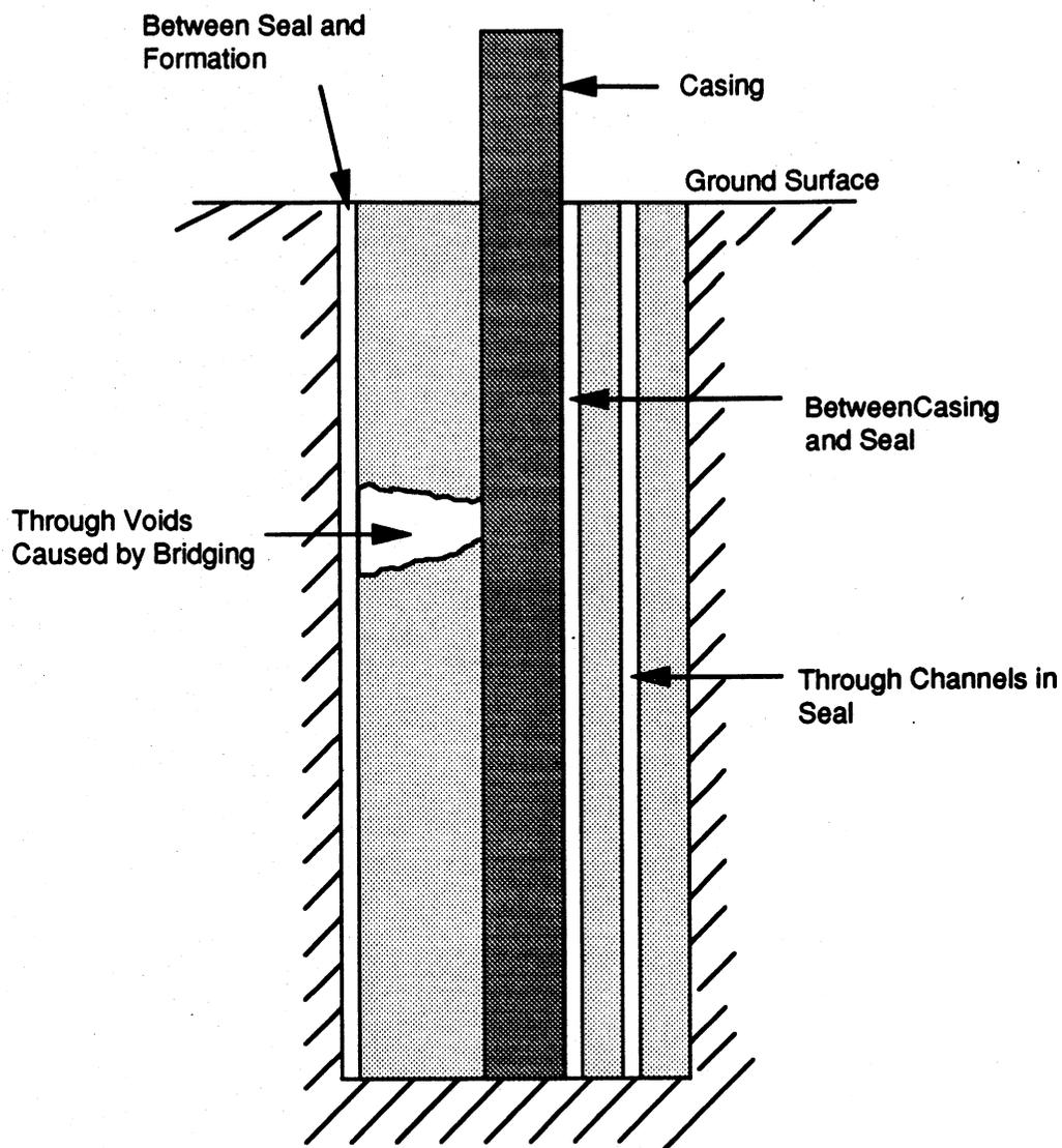
Fig. 2.1. Potential Pathways for Contaminant Transport in the Annular Space (adapted from Nielsen and Schalla, 1991)
