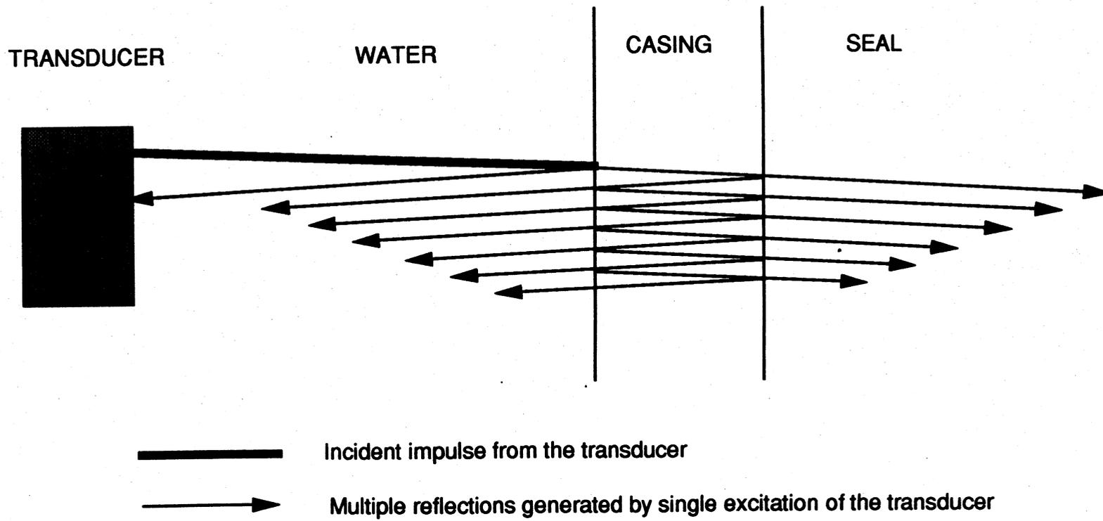
Fig. 4.4. Wave Sequences Generated in Model Borehole Tests
