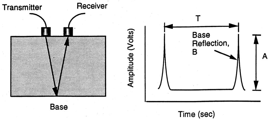
(a) Intact Test Specimen
