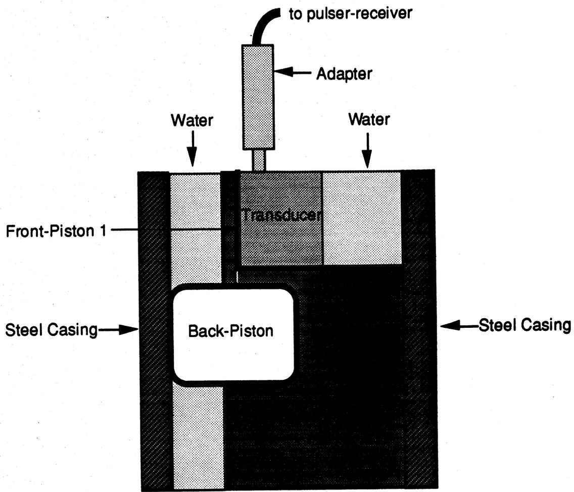
Fig. 4.2. Pressurized Probe in the Casing
