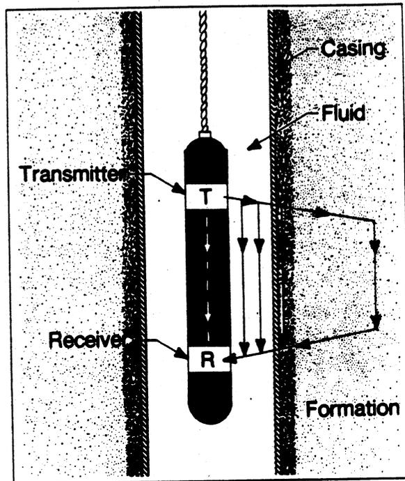
Fig. 2.4. Cement Bond Logging Tool and Wave Paths
