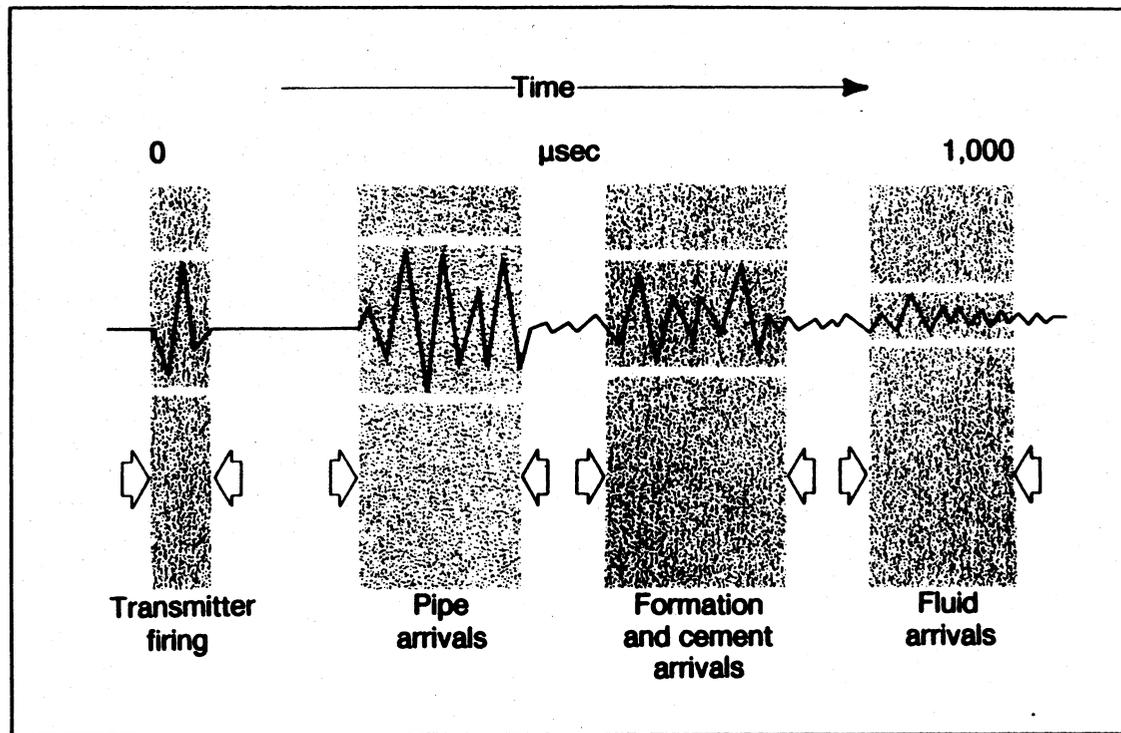
Fig. 2.5. Composite Waveform Obtained In Cement Bond Logging (after Driscoll 1986)
