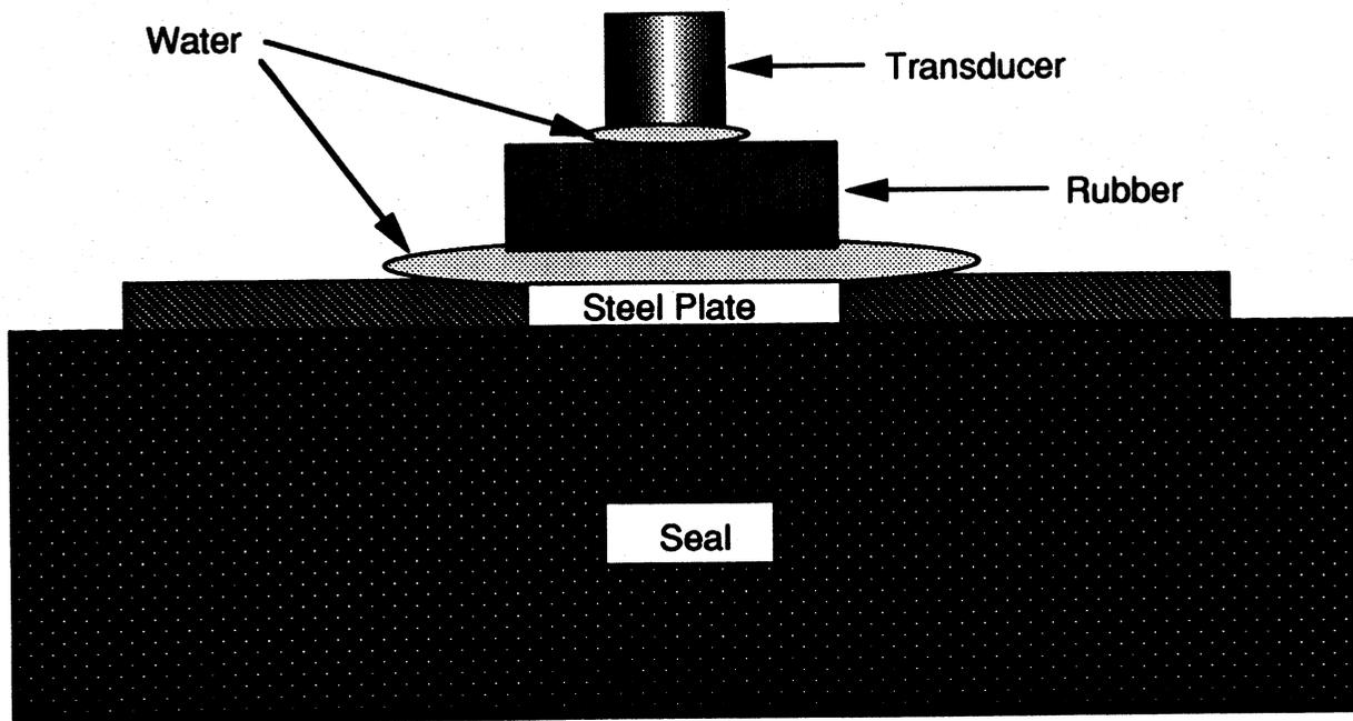
Fig. 3.1. Arrangement of Materials Used in Planar Tests
