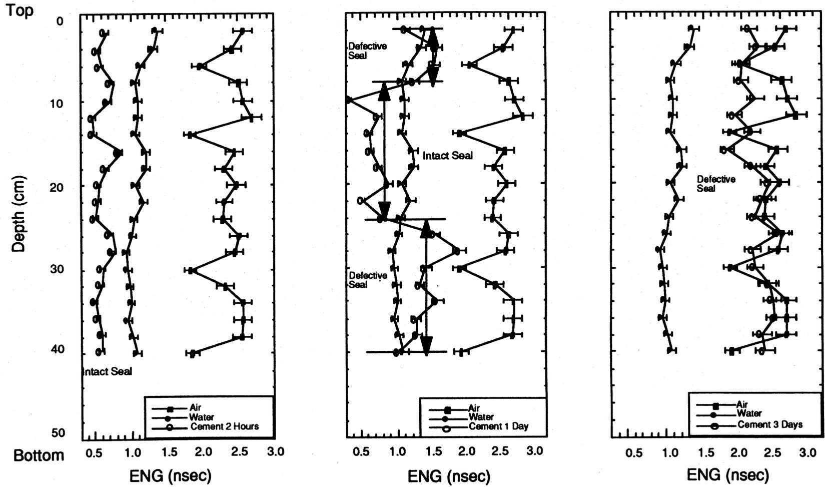
Fig. 4.10. Tests with Air, Water and Neat-Cement in the Annular Space
