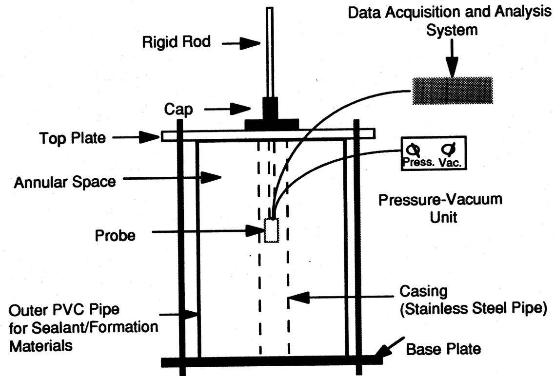
Fig. 4.3. Laboratory Borehole Model with Probe
