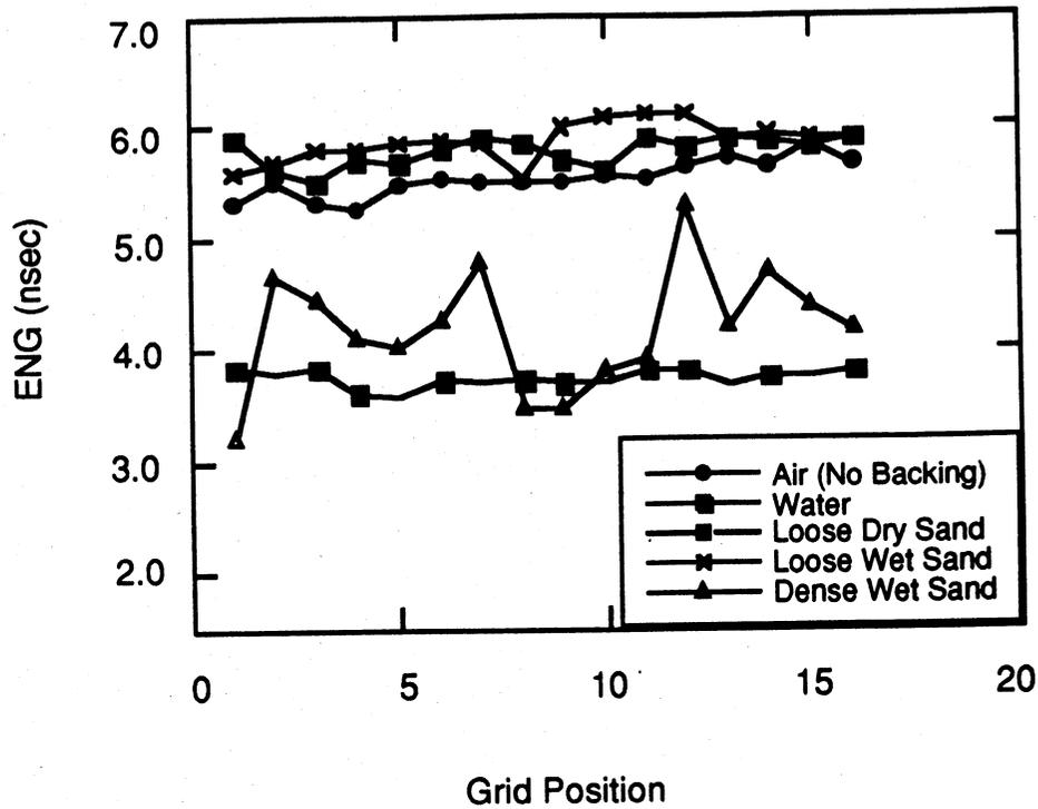
Fig. 3.11. Comparison of Planar Tests Conducted with Air (no backing), Water, Loose Dry Sand, Loose Wet Sand, and Dense Wet Sand
