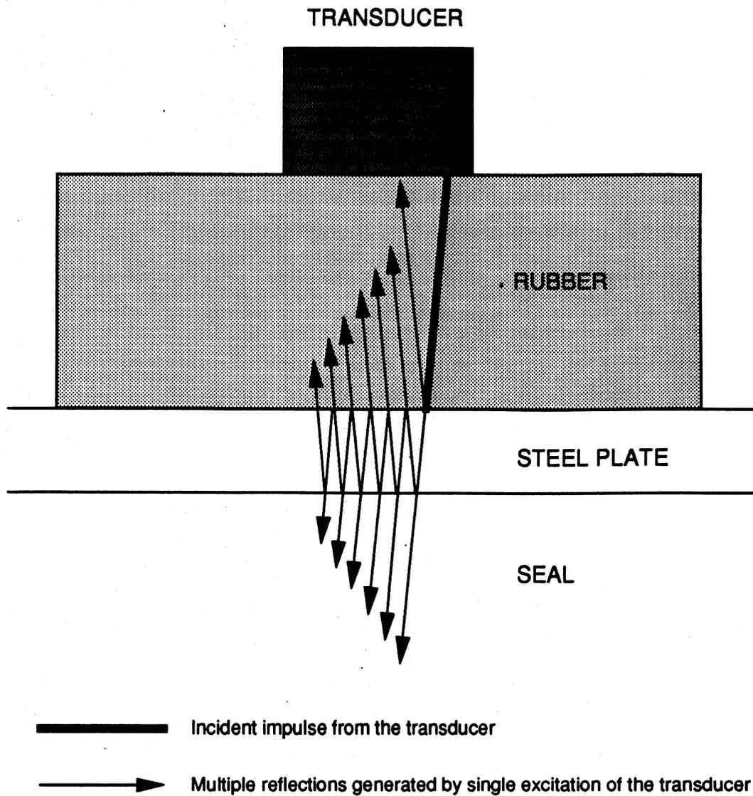
Fig. 3.5. Wave Sequences Generated in Planar Tests
