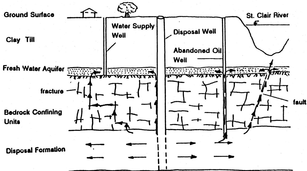
Fig. 2.2. Potential Paths for the Upward Migration of Liquid Industrial Waste (after Lesage et al. 1991)
