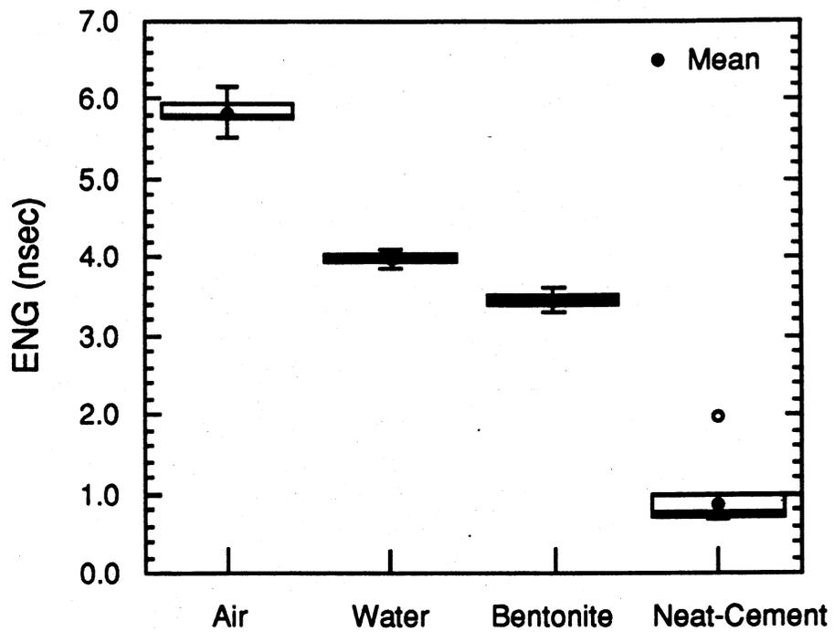
Fig. 3.8. Box Plot of ENG for Different Materials Tested in Planar Arrangement
