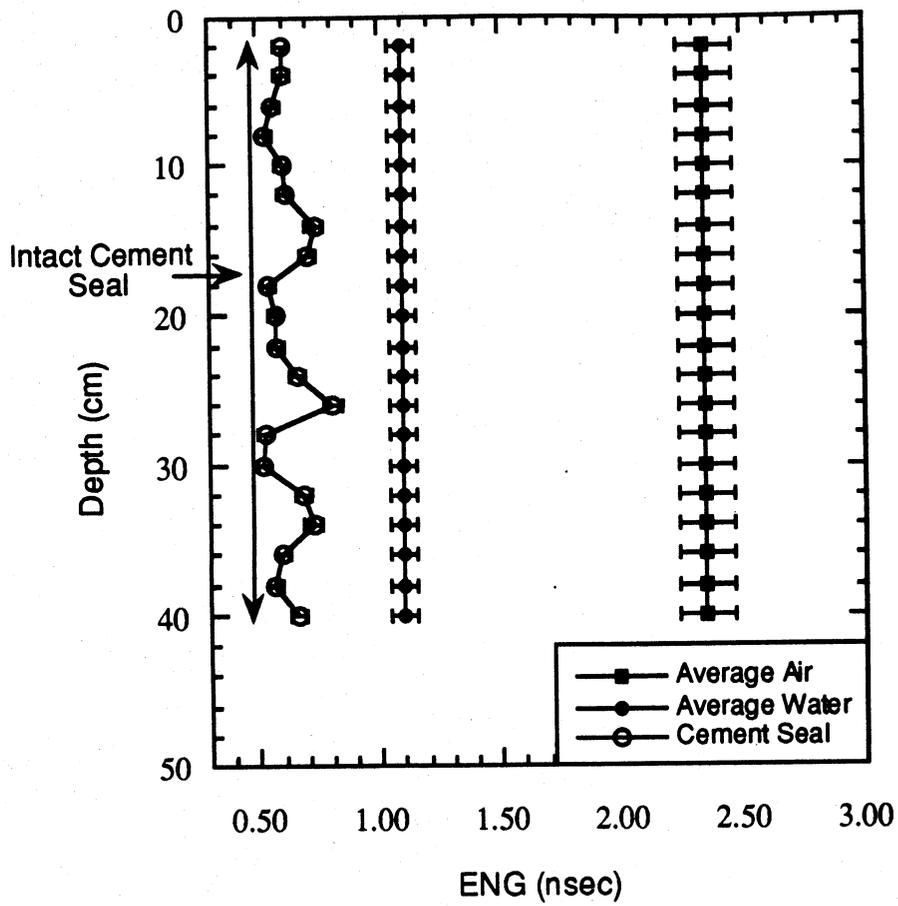
Fig. 4.7. ENG Profiles for a Sealed Casing, Average Water Backing, and Average Air Backing
