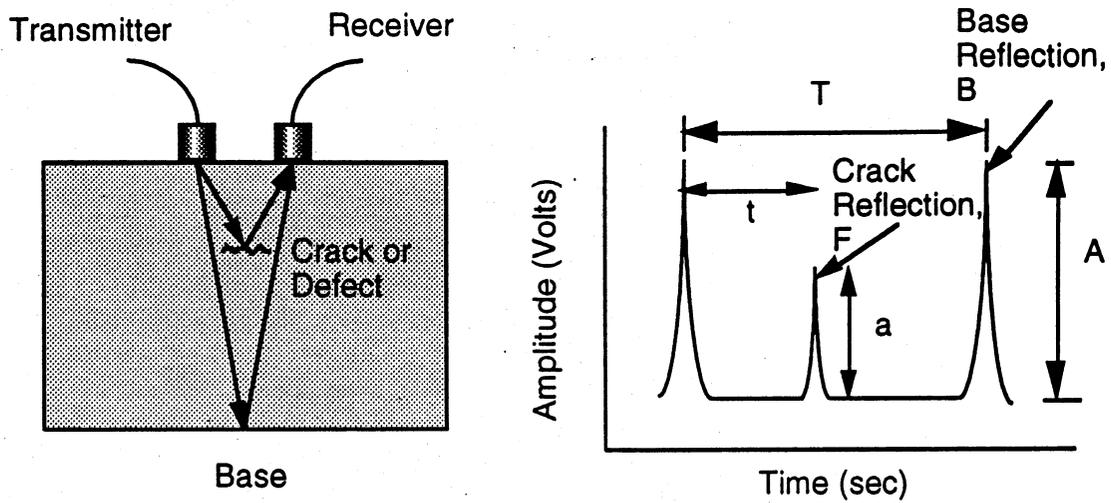
(b) Test Specimen with a Crack or Defect
