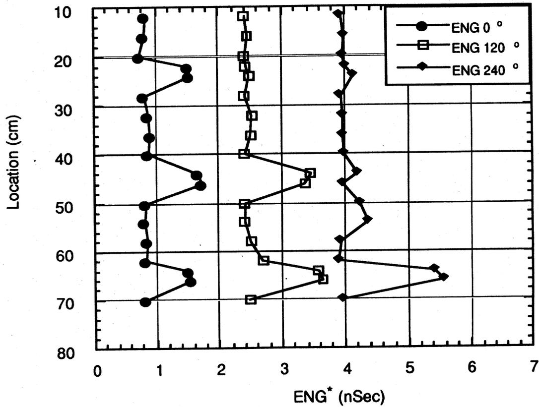
\* ENG is similar in all of the tests conducted in different directions. 1.5 nSec is added to the ENG obtained from 120° tests, 3.0 nSec is added to the ENG obtained from 240° tests to provide a clear representation of the results from all three tests on the same graph.
