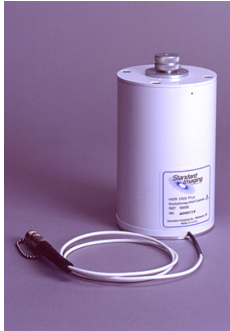
Figure 3.7: An image of the HDR1000 Plus well chamber manufactured by Standard Imaging. [Image reproduced from: https://www.standardimaging.com/ ]
