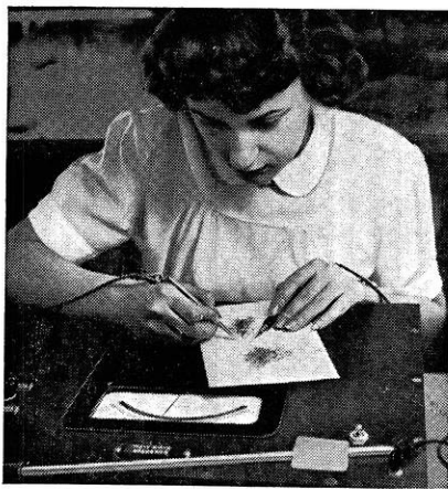
At Western Electric's Allentown (Pa.) Plant hundreds of minute thermistor components are electrically tested and sorted every day. The basic component, an oxide, has a large negative temperature coefficient of resistivity.
