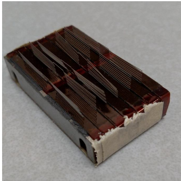
Fig. 62: Short section of assembled MTM structure using SS meander elements and painted spacers.
