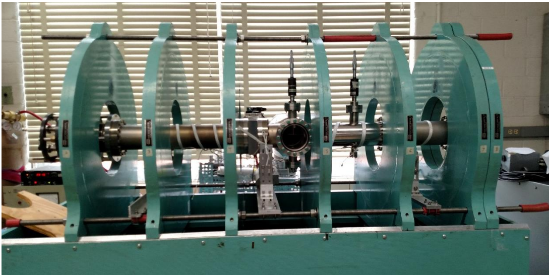
Fig. 64: Vacuum chamber setup used for all experimental hot tests discussed in this dissertation. The vacuum chamber is a 4" cylindrical tube encompassed by large electromagnets. The electron pencil beam used for the experimental tests travels from left to right in this configuration.
