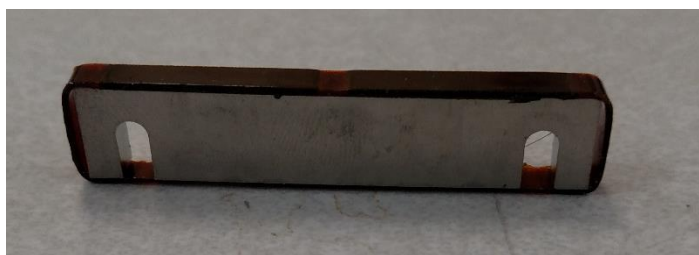
Fig. 61: A spacer element with five alternating layers of Kapton tape and graphite paint.
