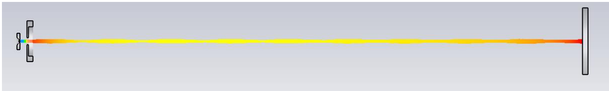
Fig. 76: Electron gun simulation showing the full simulation showing the full travel distance of the confined electron beam, anode, cathode, and collector. The beam ripple in this simulation is very low.
