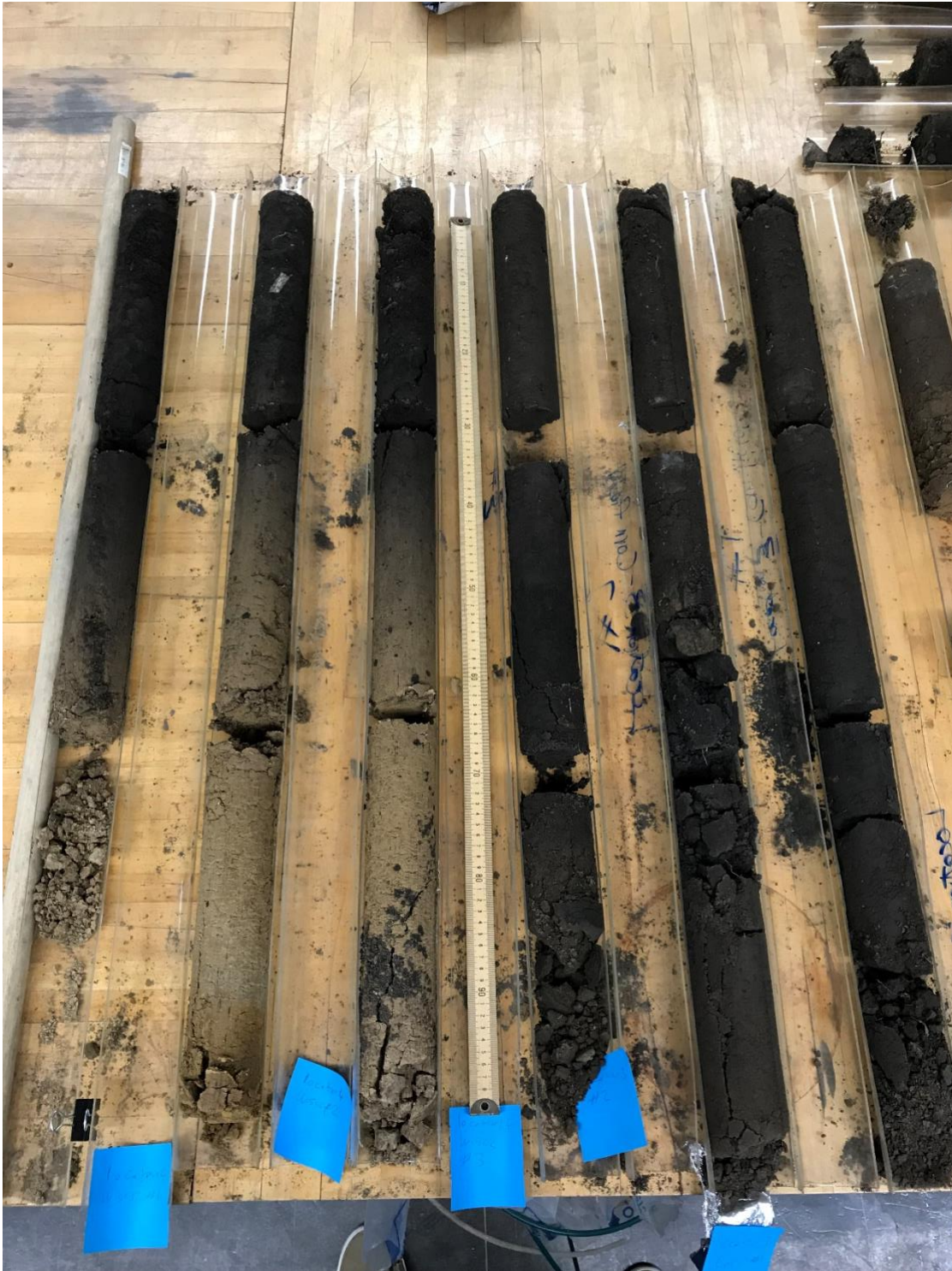
Figure S.4. An example of intact core samples divided into three depths 0 – 30 cm, 30 – 60 cm, and 60 – 90 cm depths, used in chapter 2 and chapter 3.
