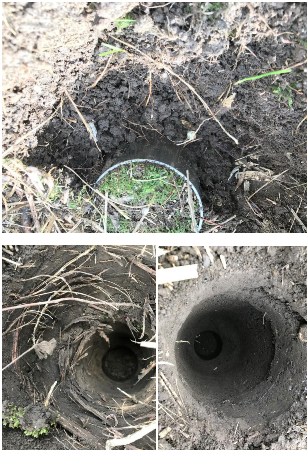
Figure S.7. An example of metal intact core sampling and profile view from surface 0 – 5 cm and 30 – 35 cm depths in a woodland (left down), grassland (top), and cornfield (right down), used in chapter 2 and chapter 3.
