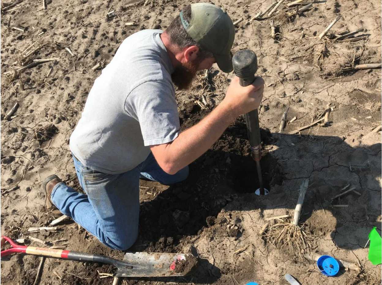
Figure S.12. An example of metal intact core sampling from surface 0 – 5 cm depth in Arlington, Wisconsin, used in chapter 4.
