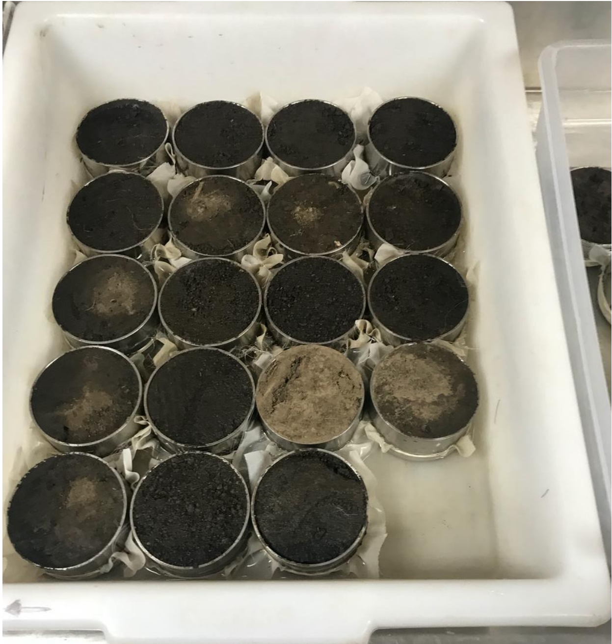
Figure S.8. An example of saturation of metal intact core samples of woodland, grassland, and cornfield, used in chapter 2 and chapter 3.
