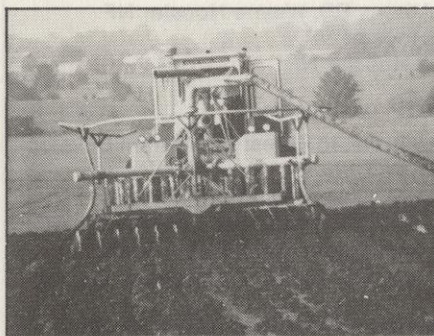
Sludge was pumped through a rubber hose and disked into the spoils of Palzo. (Photo by Charles Gill; RO-OI)
