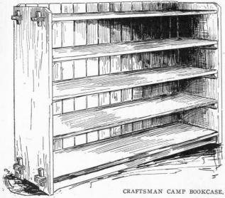
nishes a brace that greatly strengthens the construction. The back of the bookcase is made of V-jointed boards 4 inches in width. The tongue and groove construction of these boards is shown in detail C. There is no necessity to use glue in joining them, as the boards fit closely together and are screwed to the top and bottom of the case by means of ordinary screws inserted from the back. These screws can be removed and replaced at any time in taking the bookcase apart. The boards should be
