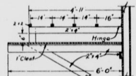
DETAIL OF ROOSTS
