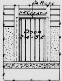
-ELEVATION OF SLIDING DOOR - (Interior View)
