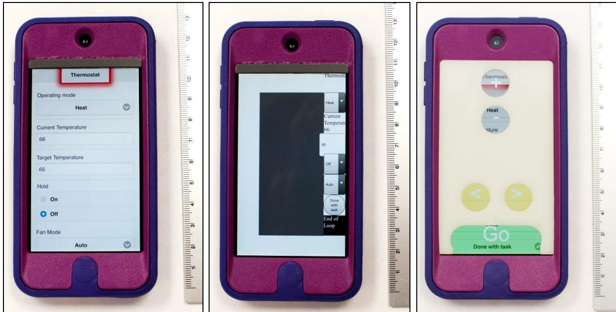
Figure 4-2. Photographs of List, Loop, and Panel interfaces. All of the interfaces were on an iPod Touch PAUI device. The List and Loop interfaces were operated with touchscreen gestures. The Panel interface has a plastic panel overlay that tactilely delimits where the five on-screen buttons are that are used to navigate and operate the interface. The Button interface (not shown) added physical buttons in the location of each hole in the plastic panel of the Panel interface, but the interface usage was exactly the same. Rulers in the figure are marked in cm.
