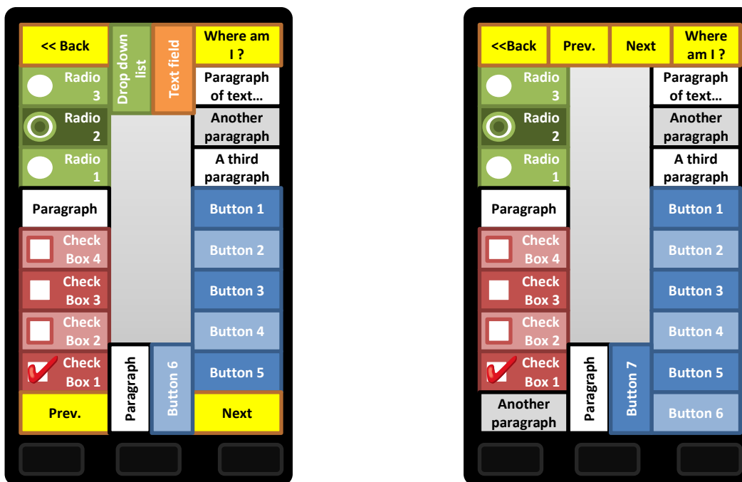
Figure D-3. Two possible alternatives for dedicated controls. Dedicated controls in this figure are yellow and are labelled: “Where am I?”, “Back”, “Next”, and “Prev.” The figure on the left shows the dedicated controls in the corners. Notice that they interrupt the circular flow of the circular list of elements. The figure on the right shows the dedicated controls all at the top of the screen in a toolbar-like arrangement.
