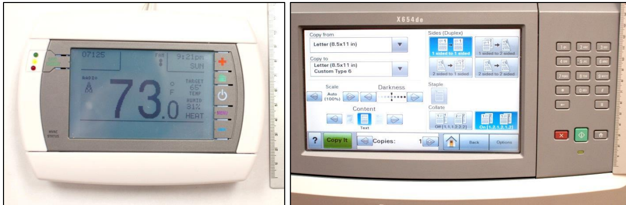
Figure 5-1. The thermostat and controls on the copier. Both systems had a touchscreen and physical buttons. Rulers in the photographs are marked in cm.
