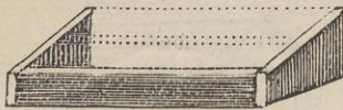
ENTRANCE-BOARD BEFORE THE CLAPBOARDS ARE PUT ON, THE DOTTED LINES SHOWING WHERE THEY GO.
