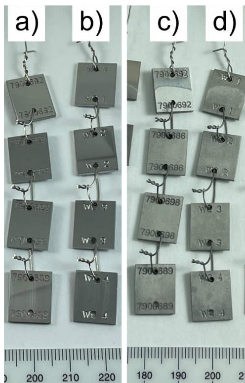
Figure 56. SEM images for (a)(c) 316H substrate and (b)(d) 16-8-2 weld specimens (a)(b) before and (c)(d) after exposure to FLiNaK for 500 hours at 700 °C in pyrolytic boron nitride (PBN) capsules.
