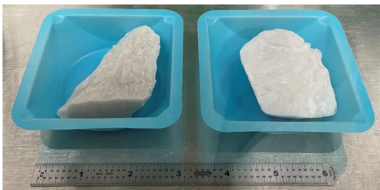
Figure 15. FLiNaK salt before (left) and after (right) purification. The white color generally indicates a higher purity salt.
