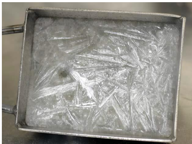
Figure 13. FLiBe salt solidified in a nickel tray after being poured from a nickel transfer vessel [105], [116]. The large dendritic structures are a manifestation of the high purity of the salt.
