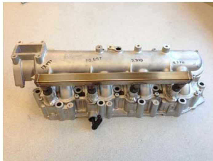
Figure 3-5 Modified GM 1.9L intake manifold and port fuel injection system
