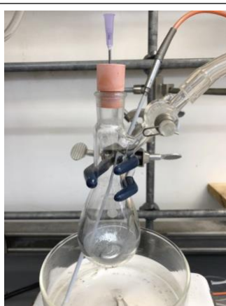
Image 2. Addition of LiCl, aryl chloride, and zinc flake.
