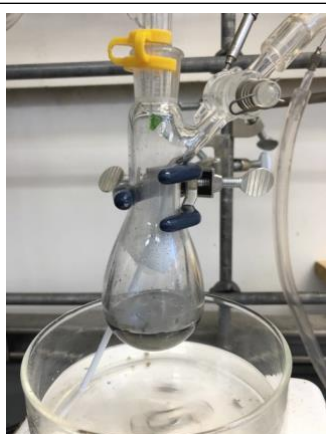
Image 4. Reaction after addition of the catalyst solution via syringe under N_2 .
