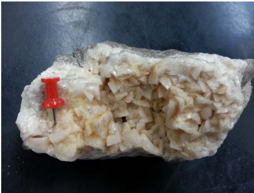
Figure 1.1.2 Saddle dolomite with curved crystal faces is very common in natural dolomite. This sample is from the mineralogy lab collection at UW-Madison (#6229, location: near Baxter Springs, Kansas)
