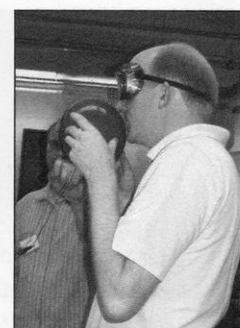
CMS PARTICIPANT TESTING MICROPHONE MADE FROM PIEZOELECTRIC STRIP AND BALLOON.
