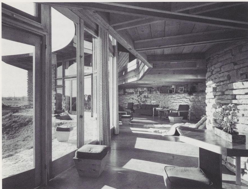
The main floor of the Solar Hemicycle from the east (kitchen) end, showing the direct-gain solar heating at work. Also apparent is the major exposed thermal mass, the open volume of the main floor, the low ceiling produced by the mezzanine level, and the open front of the mezzanine level to promote two-story thermal circulation. Copyright Ezra Stoller, ESTO. Used by permission.
