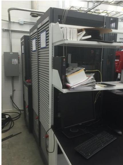
Fig. A.3: Digatron testing power units
