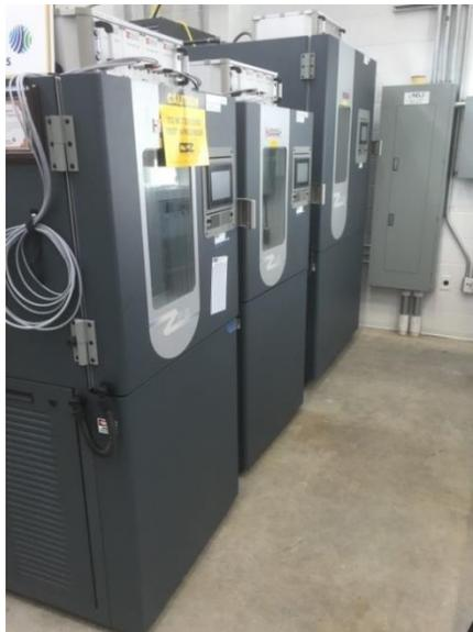
Fig. A.4: Fully-monitored thermal chambers from CSZ
