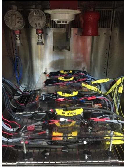
Fig. 3.2: 9-cell aging experimental setup
