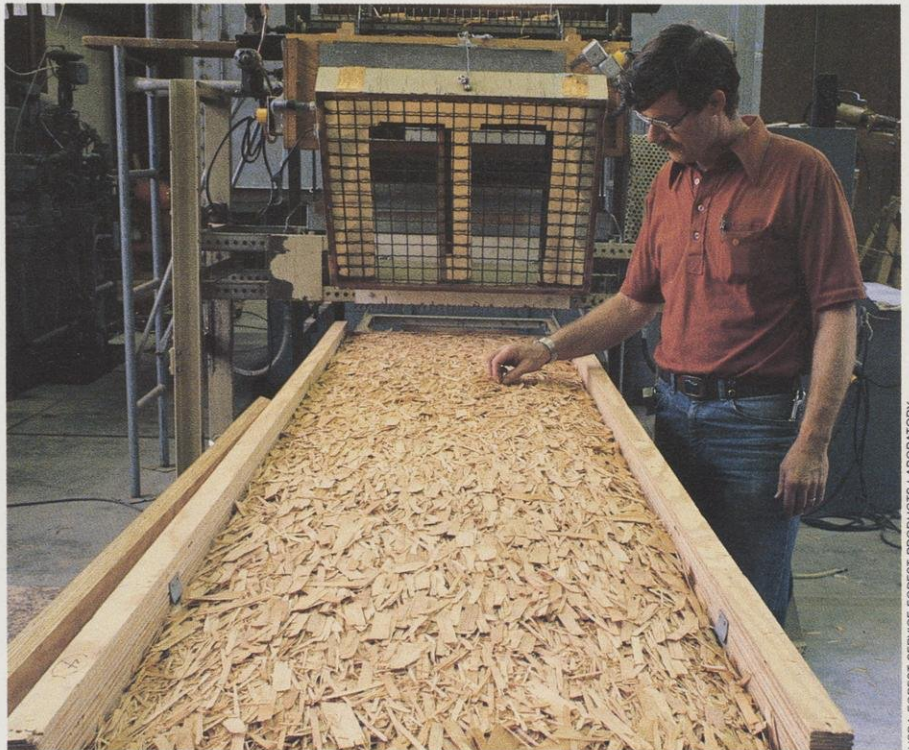
A new wrinkle: Resin-coated wood chips and flakes are injected with steam and quickly molded to form sturdy particle board and flakeboard. Instant pressure and blistering 280-315° F heat cure the adhesives, turning loose chips into solid board in less than two minutes.
