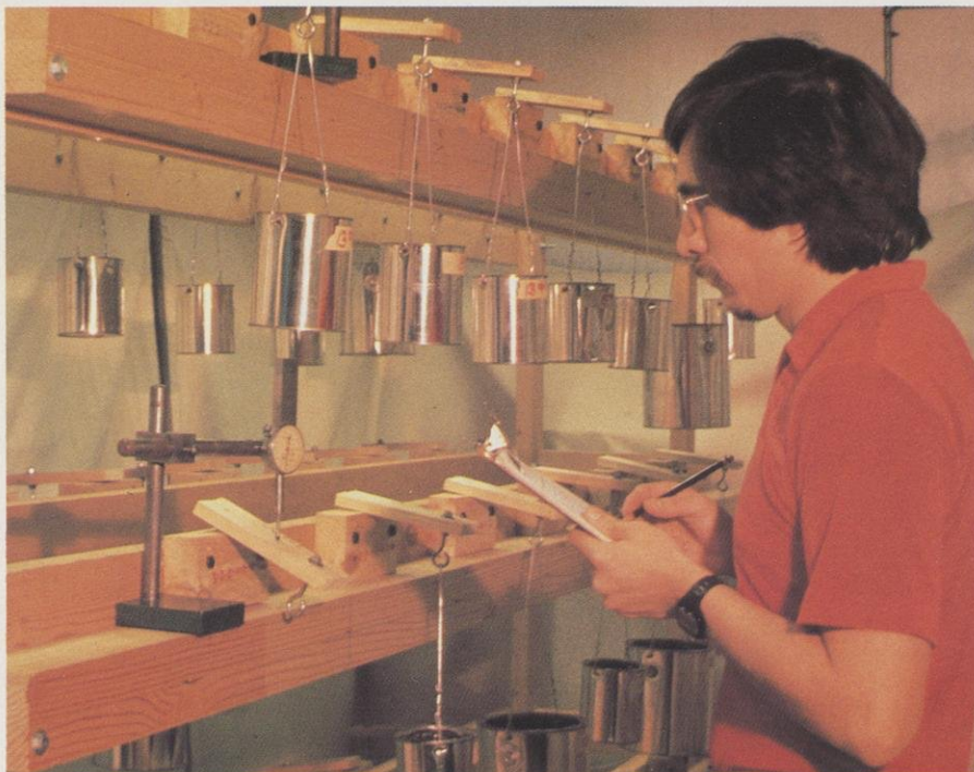
Testing the tensile strength of various types of wood and new wood products is a key to comparing product quality.
