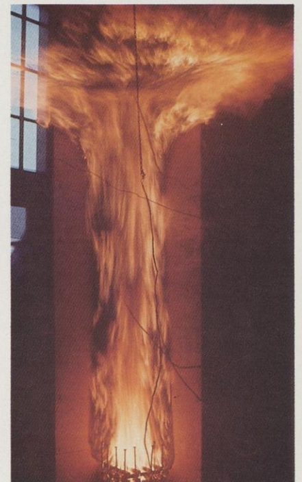
Judging wood by its cover: Wood preservatives, stains and paints get a trial by fire to prove their resistance to heat and flame.
