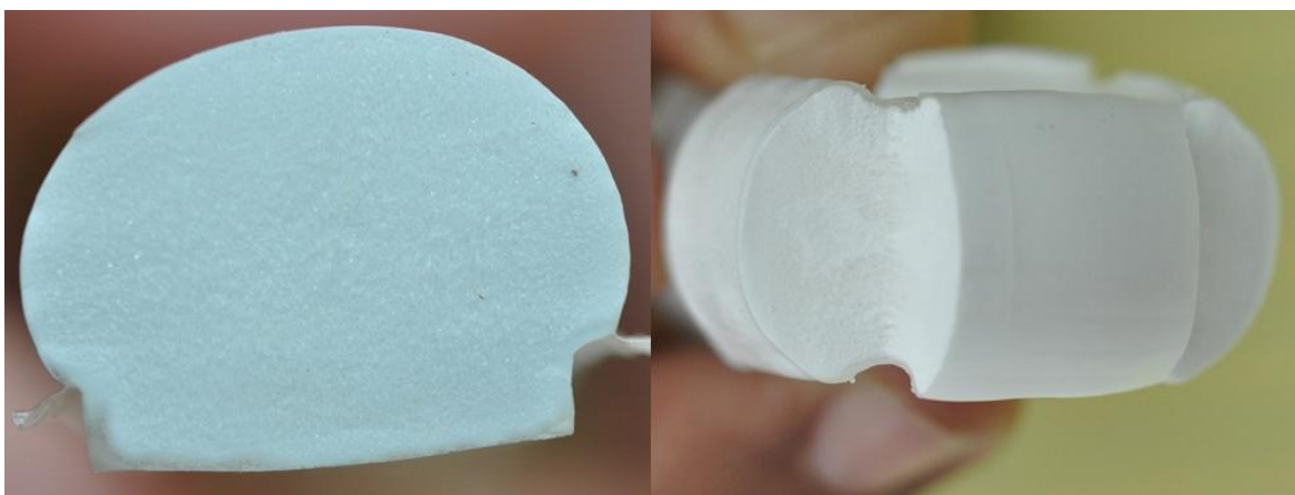
Figure 3.8. Images of the foamed cross-sections of microcellular injection molded TPU parts with a cross-linking agent.
