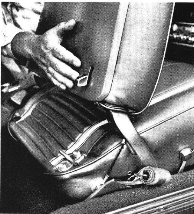
The mechanism pictured above is designed to keep the back of folding seats in place should they be hit by a rear-seat passenger thrown forward by the impact of an accident. Note the accessible, easily operated catch, designed for easy entry and exit.
