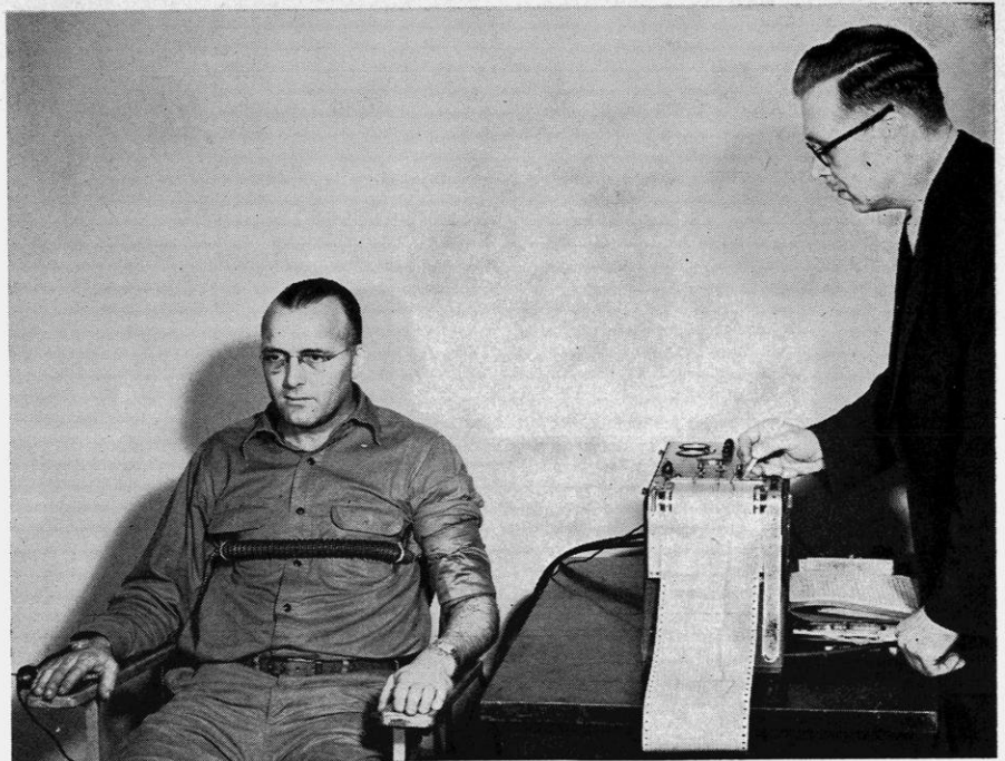
A SUBJECT undergoing a lie-detector examination in the crime lab. The device records emotional reactions, thus indicating if the person being questioned is telling the truth.
