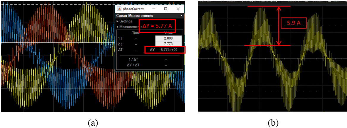
Figure 6.2-5. Motor phase current waveforms without filter (a) Simulated (b) Measured
