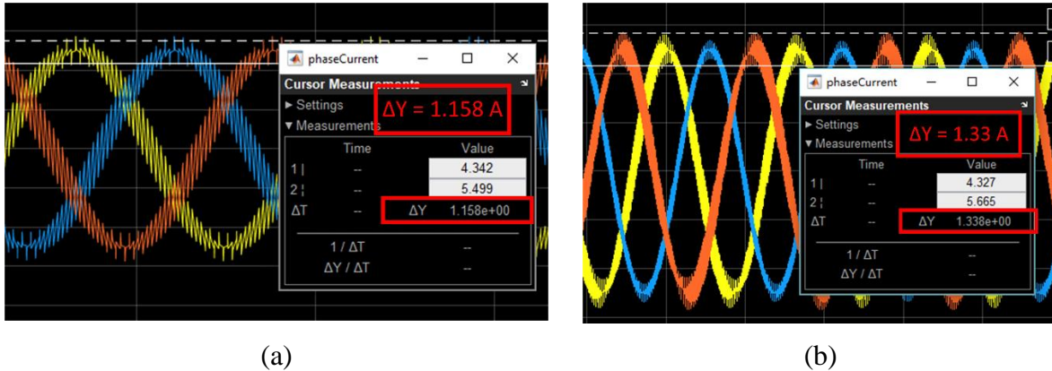
Figure 6.2-7. Motor phase current waveform with filter (a) LC sine-wave fileter (b) Inductor
