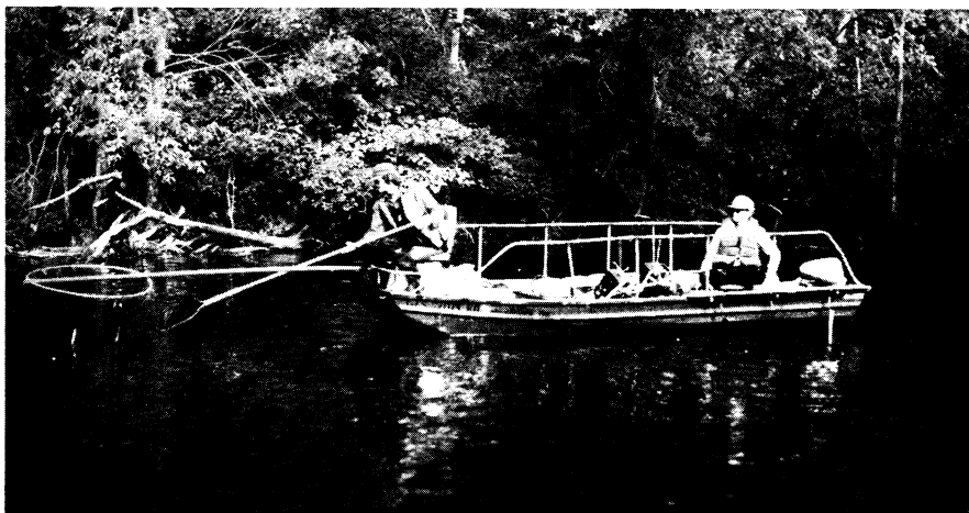
Minishocker consisting of a 16-foot flatbottom aluminum boat, 5 hp. T&J generator, and pulser control box.
