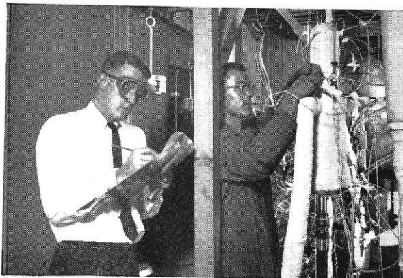
Under the close supervision of an engineer, final adjustments are made on a rig for testing an advanced liquid metal system.
