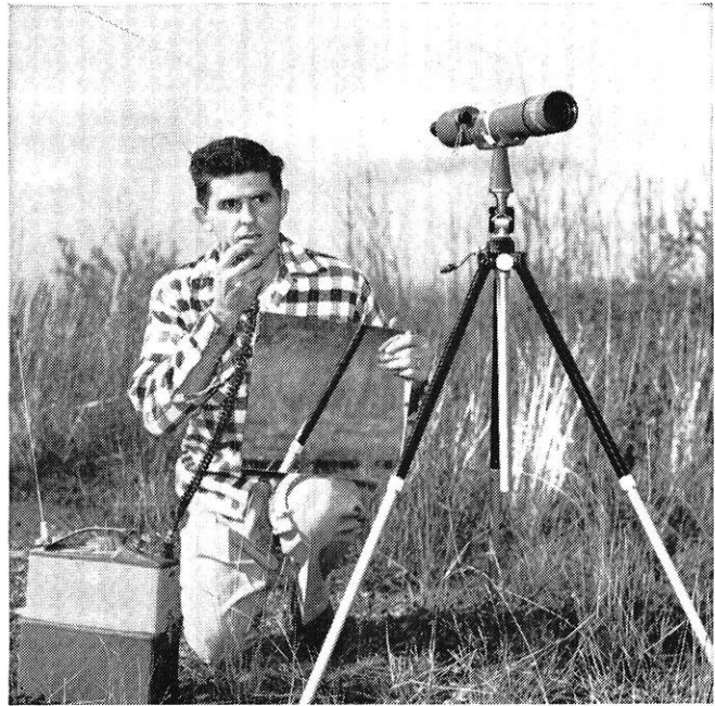
Here, Dick checks line-of-sight with a distant repeater station by mirror-flashing and confirms reception by portable radio. Using this technique, reflections of the sun's rays can be seen as far as 50 miles.
