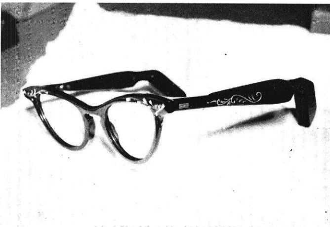
The qualitone Hearing Aid Amplifier is completely enclosed in the eyeglass frame.
