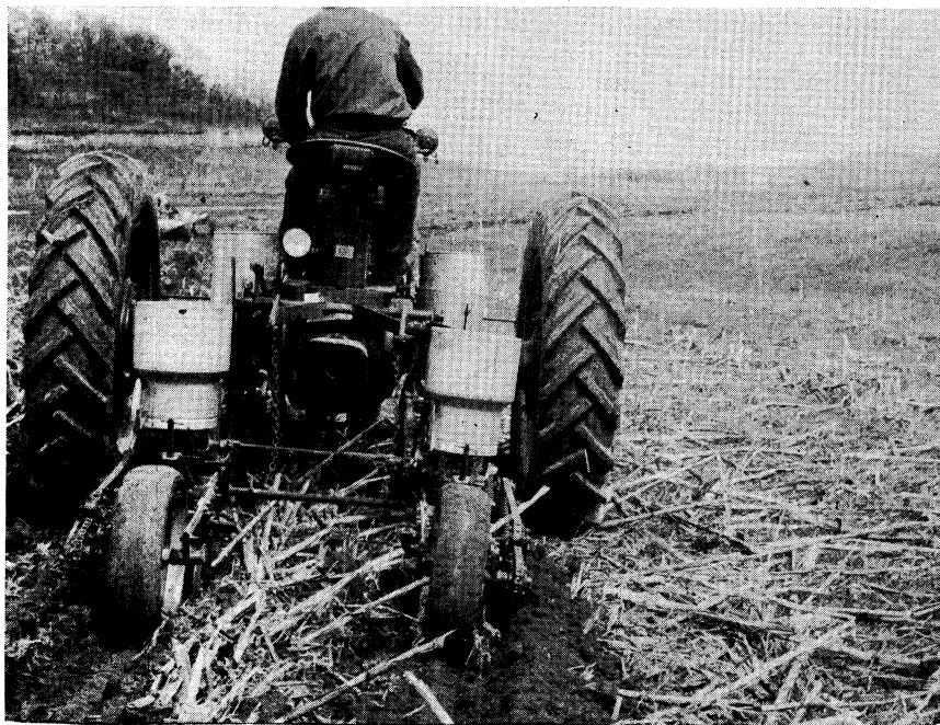
FIGURE 2. Rear view of mulch planter showing alignment of corn planter with the furrow made by the front sweeps.
