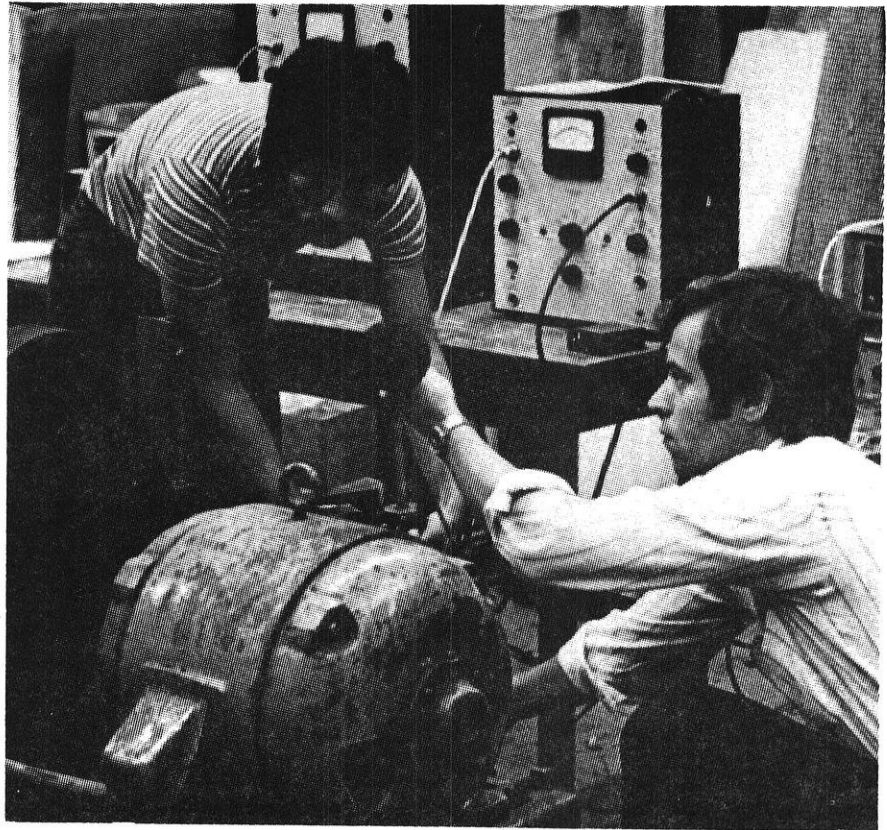
Graduate students Ray Chan (left) and Jim Yerges adjust a microphone that picks up noise produced by the wire stranding machine.
