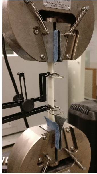
Figure 4.7: Tensile testing setup
