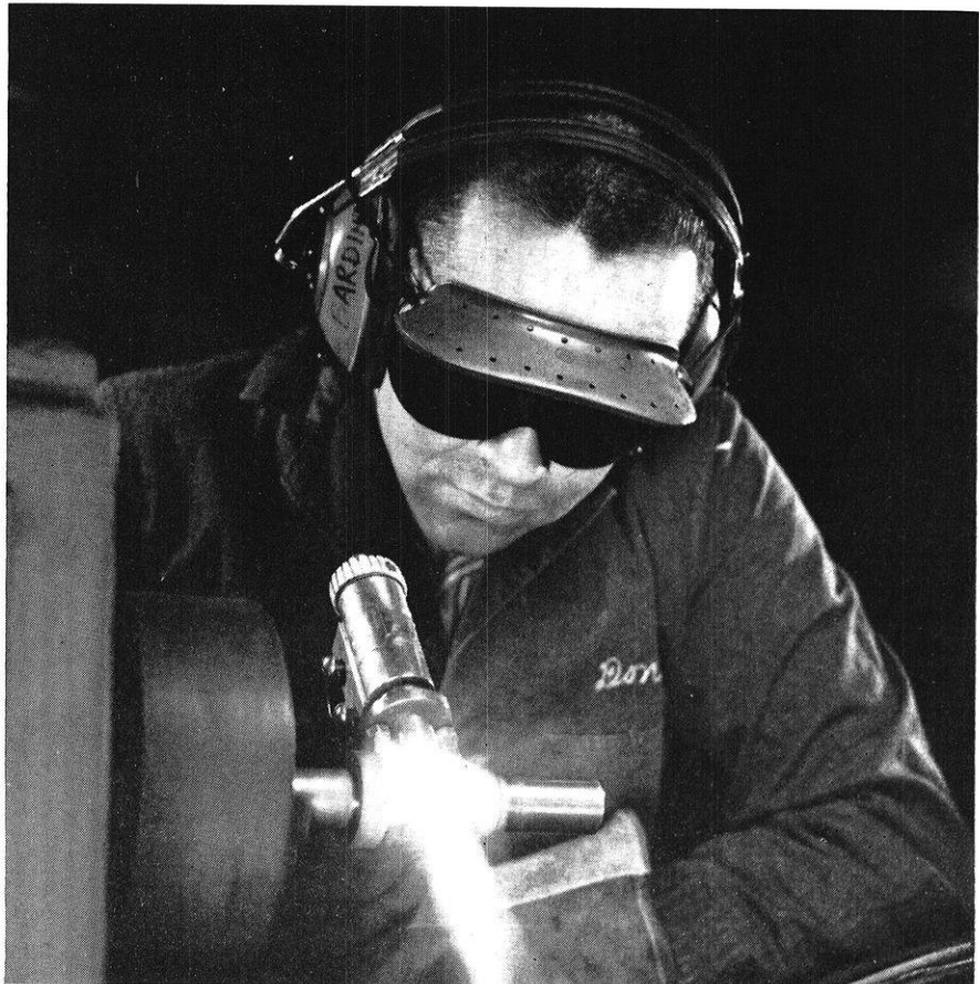
A nozzle liner for a rocket engine is made of tough tungsten with the Plasma Arc Torch. The Torch, which harnesses the highest temperatures ever used in industry; between 15,000° and 30,000° F; fabricates shapes like this by applying successive coatings on a spinning mandrel until desired thickness is reached.
