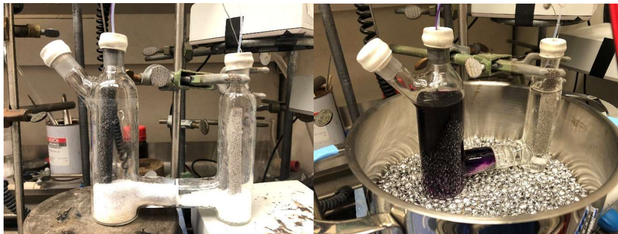
Figure C4. Left: Large scale divided cell batch assembly prior to addition of solvent. Right: Large scale divided cell batch assembly 5 minutes into electrolysis.
