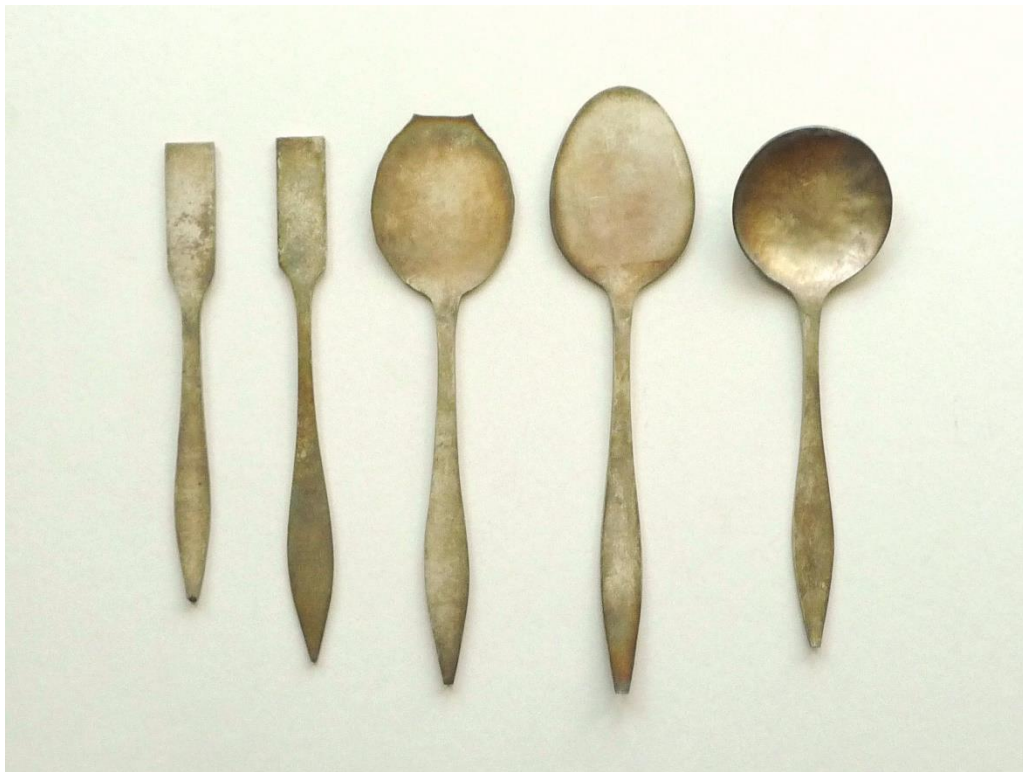
Figures 1.15 and 1.16. Ladle Forging Stages . Image sources: Broadside No. 1, Roysher Collection and Hudson Roysher Electronic Archive.
