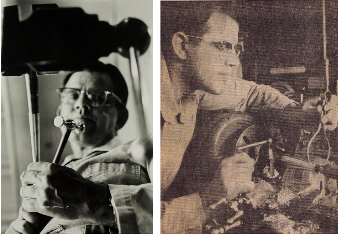
Roysher Forming Candelabrum Leg on Ring Mandrel. Image source: Binder 4, Roysher Collection.
