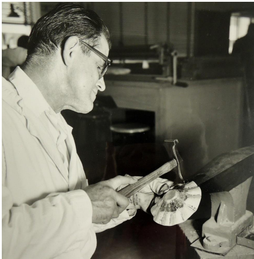
Figure 1.20. Roysher Raising Silver . Image source: Binder 4, Roysher Collection.
