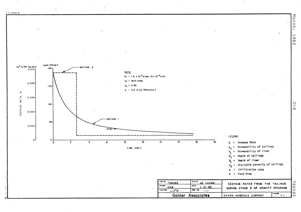
Method 1 shows the seepage rate decreasing to 25 gallons per minute  $(0.0016~\text{m}^3/\text{s})$  in about 7 years after the start of the second stage. This corresponds to 95 percent of the decrease from the maximum of 310 gallons per minute  $(0.020~\text{m}^3/\text{s})$  during the first stage to 10 gallons per minute  $(0.0006~\text{m}^3/\text{s})$  at steady-state.
