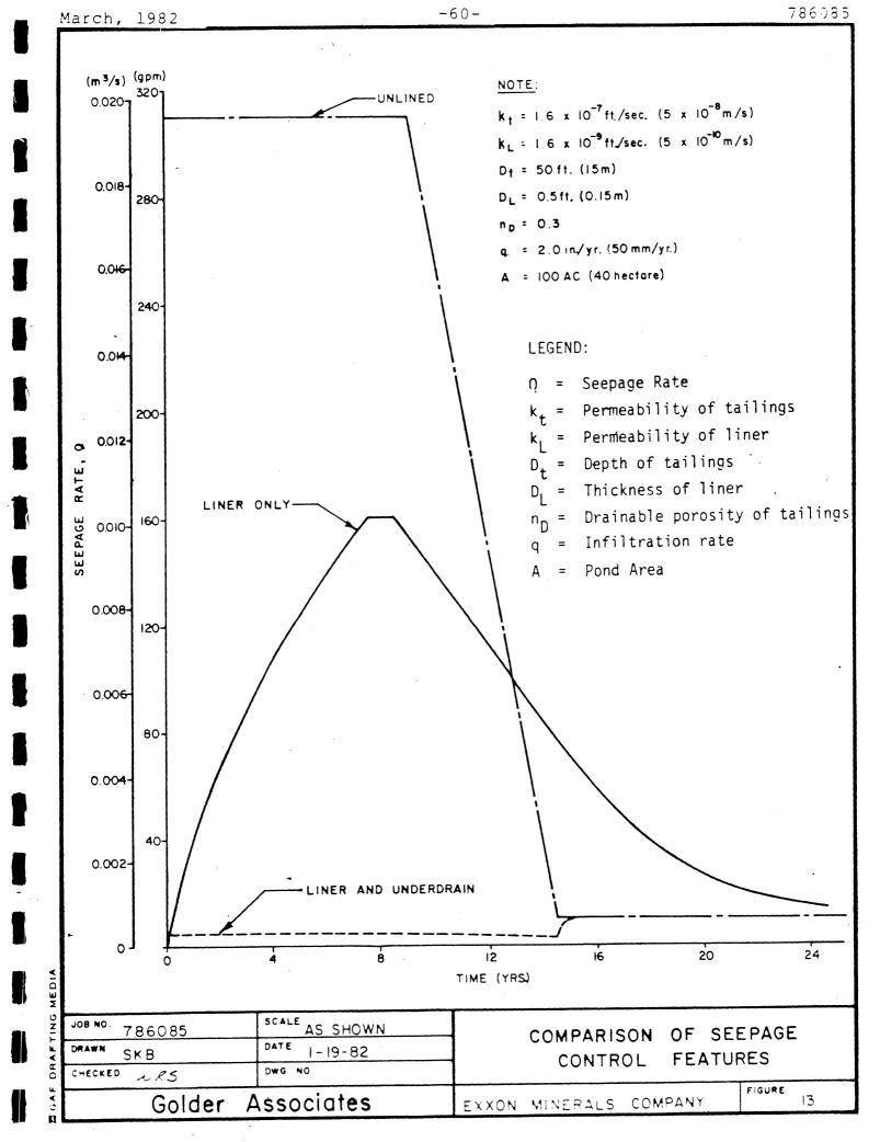
the pond with an underdrain was developed on the assumption that pumping from the underdrain continues until seepage from the tailings reaches steady-state conditions.
