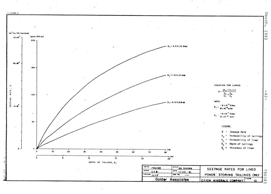
conclusion can be made for lined ponds as was made for unlined ponds. From the standpoint of minimizing seepage during operation, deep ponds with small areas are preferable to shallow ponds with large areas.
