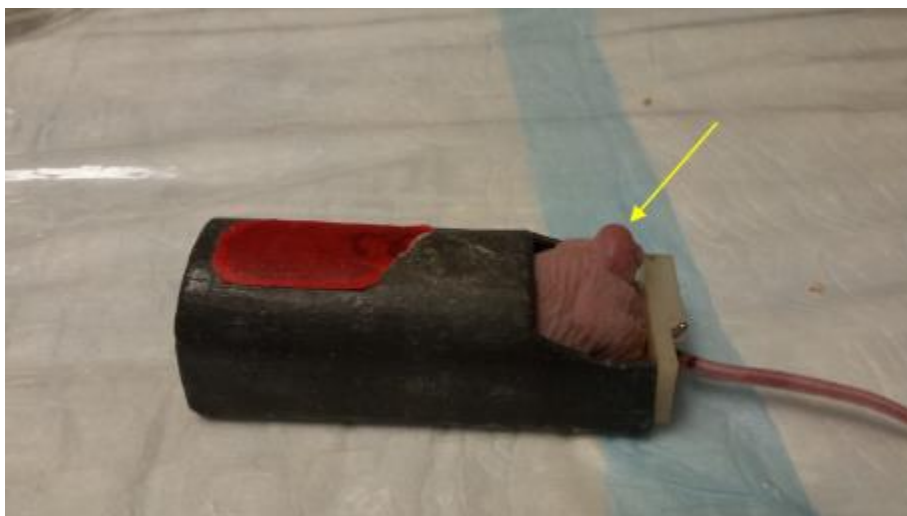
Figure 36. Irradiation setup. Mice were placed in lead shields to minimize normal tissue dose. Tumor is indicated by the yellow arrow.
