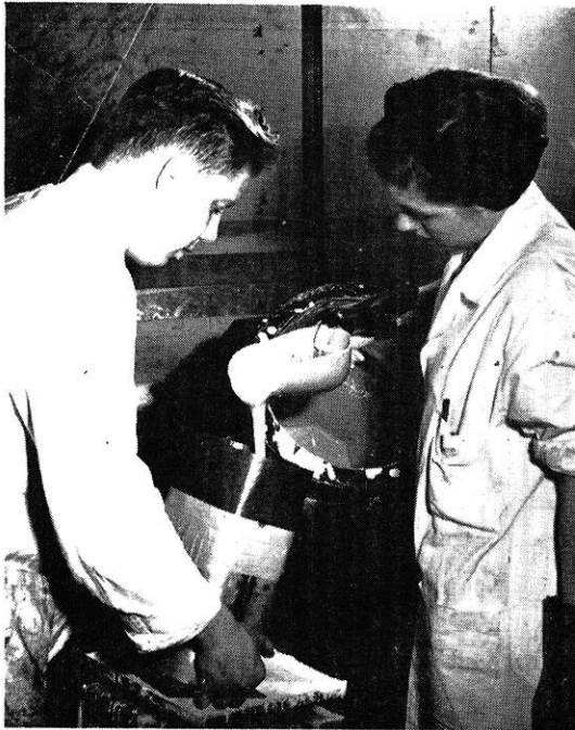
Silica and binder is poured on the patterns to form the molds.
