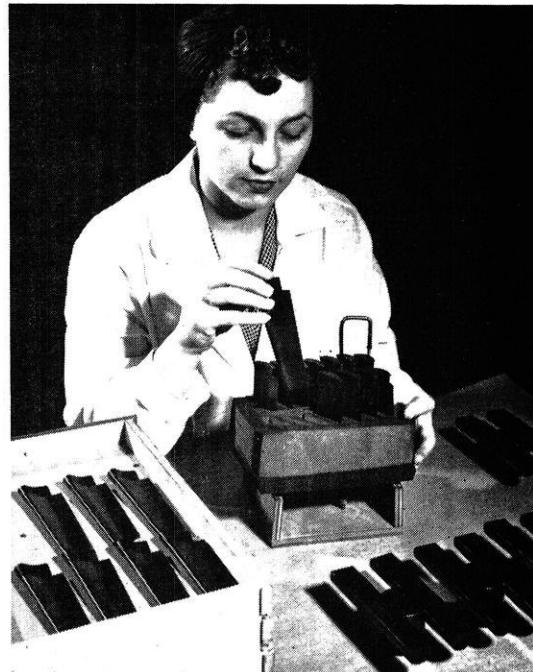
The wax pattern is placed in a "jig" and fused to a crossbar.
