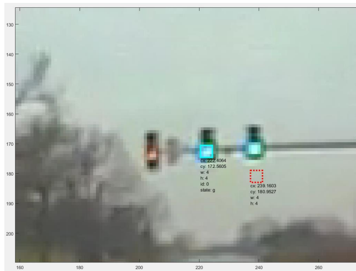
Figure 4-10 Visual interface for ground truth signal state extraction.
