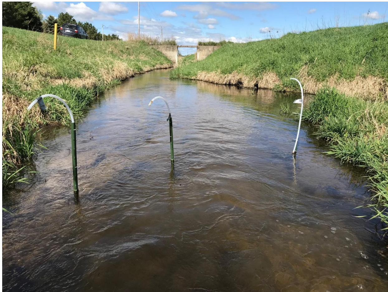
Figure 11. Example of mini-piezometer field installation at station LD5.9MD. Here three mini-piezometers were installed in a fence across the width of the ditch. This picture taken facing downstream to the west. Photo by Michael Parsen.
