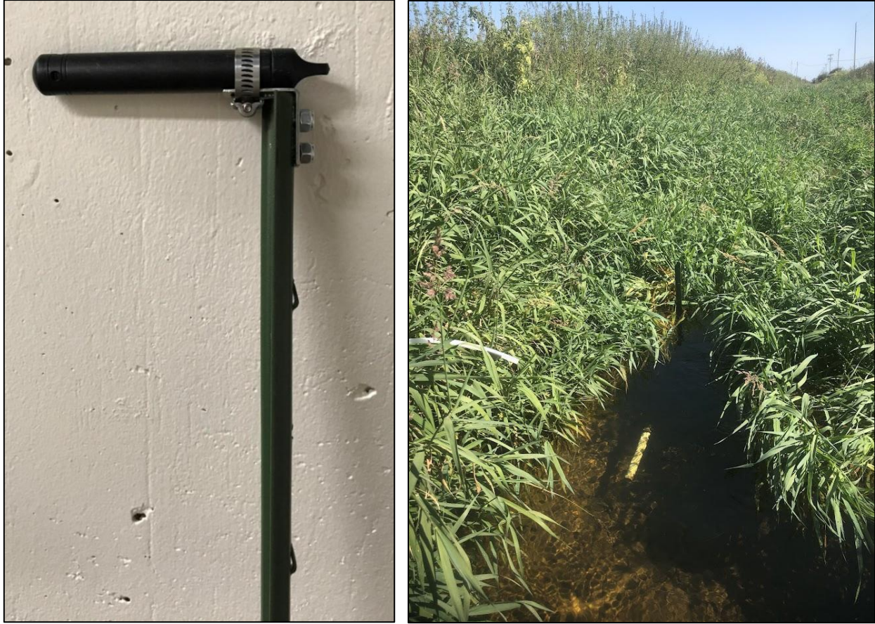
Figure 16. On left, second installation design with the conductivity probe oriented parallel and configured so the stake could be driven close to the streambed to reduce debris accumulation. Photo by Michael Parsen. On right, final installation method for Solinst conductivity probes utilizing protective stilling well in same geometry left image. Photo by William Fitzpatrick.
