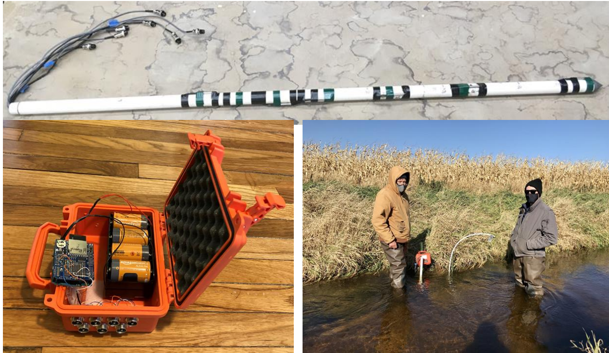
Figure 13. Upper photo, temperature probe stick used of obtaining profile measurements when driven into a streambed (Photo by David Hart). Lower left, Arduino control box used for recording data stick data (Photo by David Hart). Lower right, stick driven into streambed, with attached control box, to left of previously-installed stream-bed piezometer (long flexible tube on right) (Photo by Michael Parsen).
