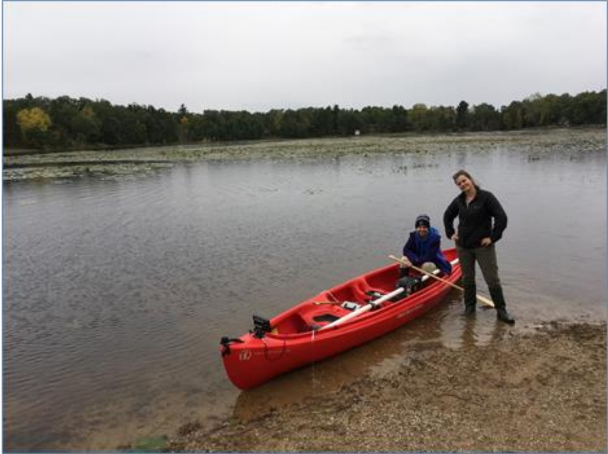
Figure 9. Canoe instrumented with EM-31 conductivity meter, depth finder, water temperature and quality instruments, and Go Pro video cameras. Photo by David Hart.
