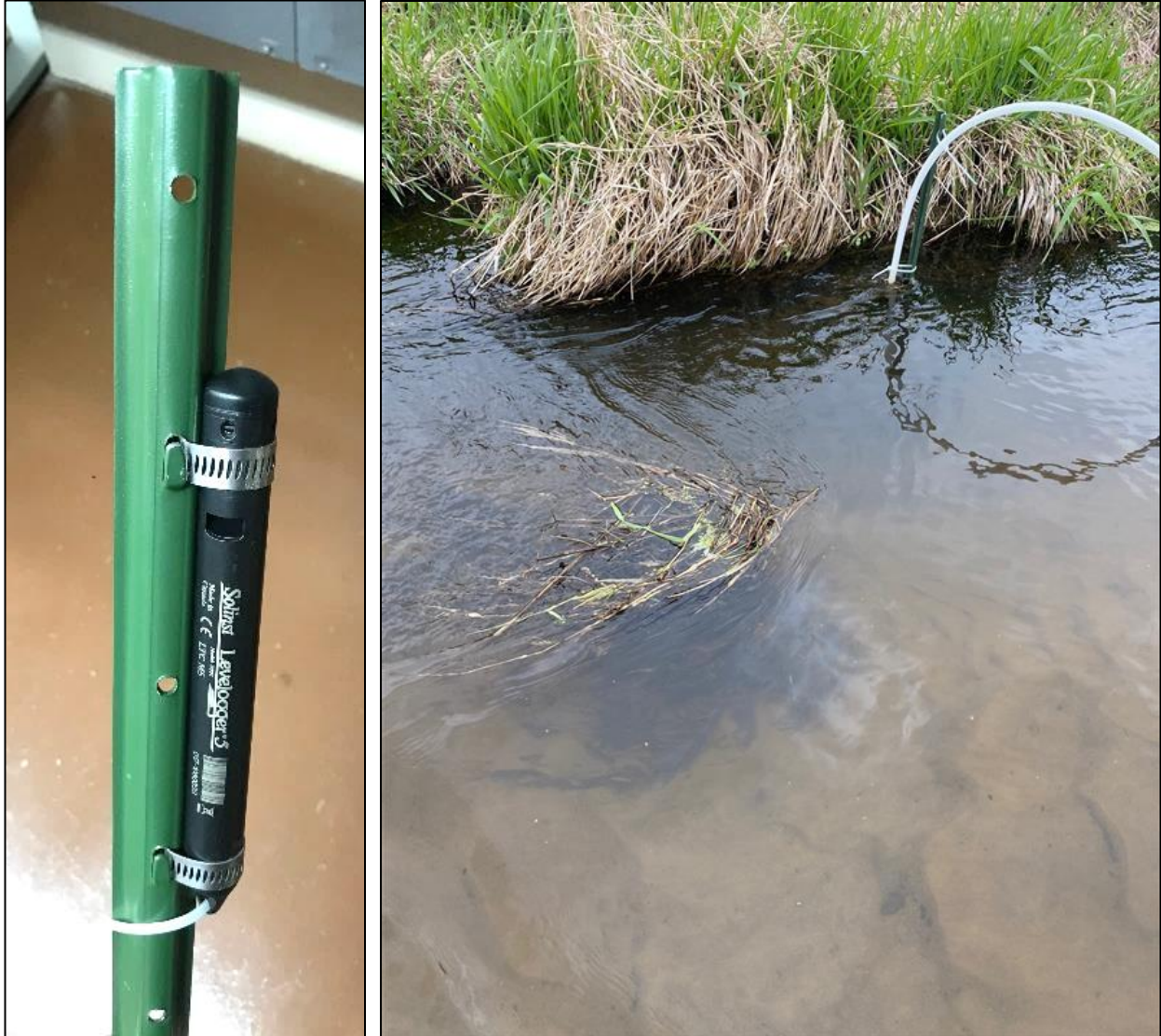
Figure 15. Left photo, original field design with Solinst conductivity probes oriented vertically (Photo by Michael Parsen). Right photo, Solinst conductivity probe deployment in Leola Ditch with accumulation of floating debris over the stake and probe (Photo by William Fitzpatrick).
