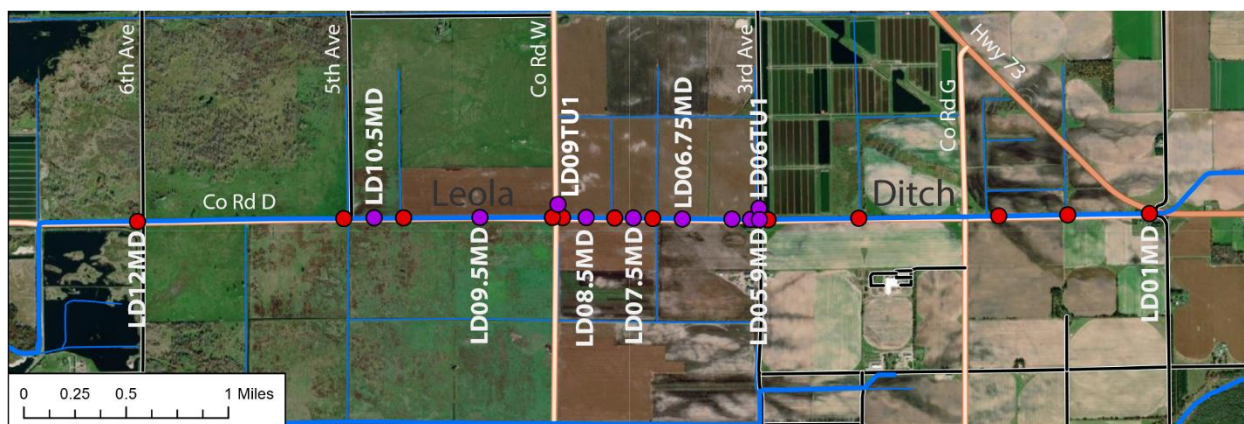
Figure 12. Overview map with satellite imagery over hillshade from 5ft LIDAR data for section of Leola Ditch monitored during this study. Thick blue lines mark larger drainages, thin blue lines represent small tributary ditches. Red circles are surface water sampling stations, purple circles are stations with mini-piezometer installations.
