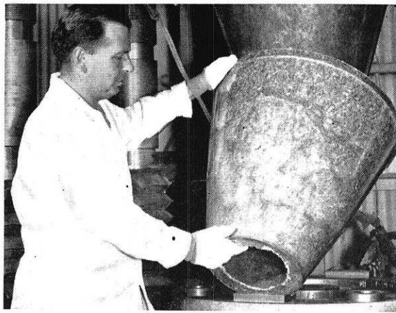
Exit cones capable of withstanding temperatures of 6000° F. represent one example of advanced engineering being performed by the Hughes Plastics Laboratory.
