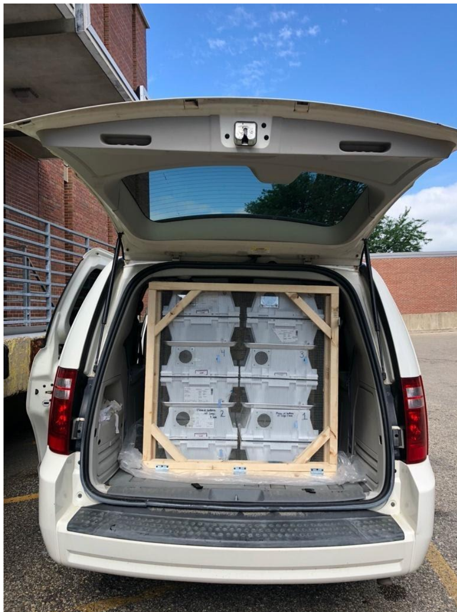
Figure 3. Final setup of the transport cages inside the minivan during transport within the U.S. The largest secondary container (shown here) held six primary containers. A smaller secondary container held three primary containers, and a tenth primary container was placed inside a commercial dog kennel cage.
