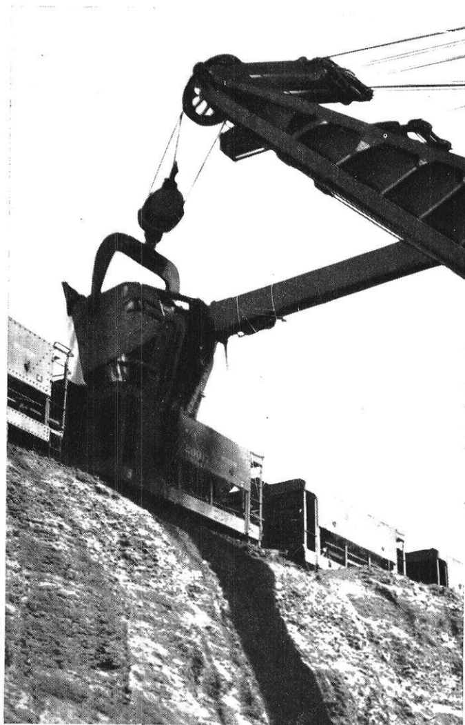
To prevent excessive wear on the teeth of a power shovel, diamond chips can be imbedded in the steel.
