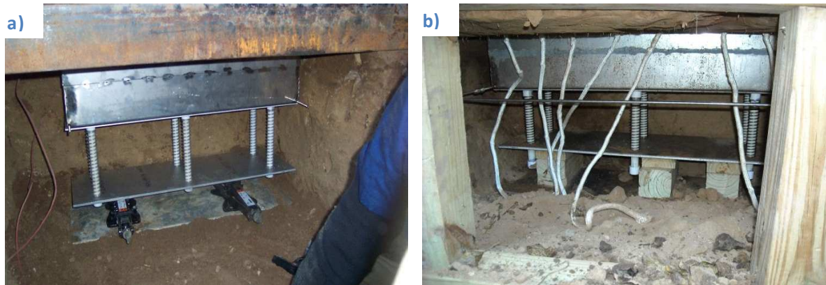
Figure B3. (a) Lysimeter and spring plate inside soil cavity with screw jacks for installation beneath. Tensiometer wires shown to the left of lysimeter. (b) Lysimeter and spring plate installed. Wooden blocks under spring plate to maintain spring force and lysimeter contact with cavity ceiling.
