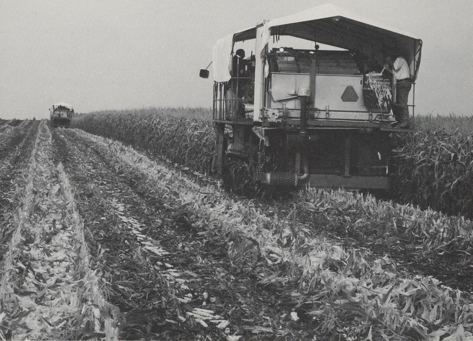
Nothin' but niblets. Byron Enterprises, Inc. developed corn harvesting equipment for Del Monte that leaves two-thirds of the wastes in the field that used to go to the cannery. Husks, cobs and silk are ground and land-spread. Machinery now cuts the kernels off 560 ears of corn a minute. The process cuts waste and drastically reduced transportation, waste disposal and wastewater management costs.
