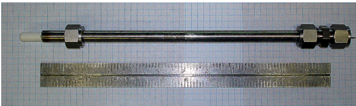
Figure 7.2: Prototype oxygen sensor 2 (P2) is shown. The YSZ crucible is epoxied in an eleven-inch stainless steel tube and a copper powder reference electrode is sealed within the probe tip.
