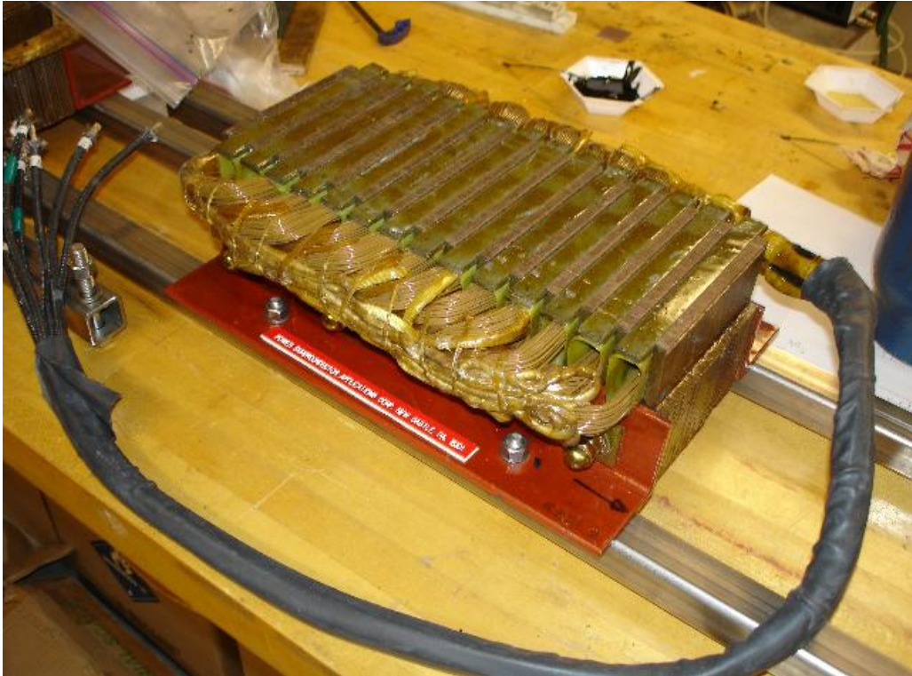
Figure 4.2: This figure shows one of the FLIPs before it was mounted to the loop. Notice the large wire coils responsible for the traveling magnetic field, which induces the eddy currents in the liquid sodium.
