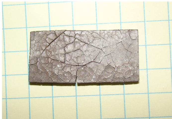
Figure 6.9: This figure shows full-fired McDanel alumina after only 100[hr] in 390[C] liquid sodium. The length of each square in the grid shown is 1/4'' .
