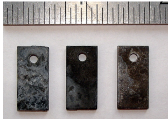
Figure 6.15: 416SS substrates after 200[hr] in liquid sodium. Testing stopped after coating began to flake from surface.
