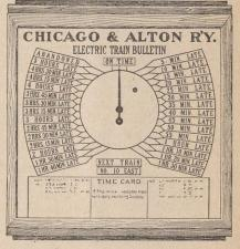
the depot. All bulletins in the waiting rooms and in the hotels, register precisely similar at one and the same instant. The operator indicates on the bulletin the number of the train next due to arrive and the time of its arrival. The machinery is similar to a telegraph instrument controlled by a telegraph key, and simple enough to be worked by a child.
