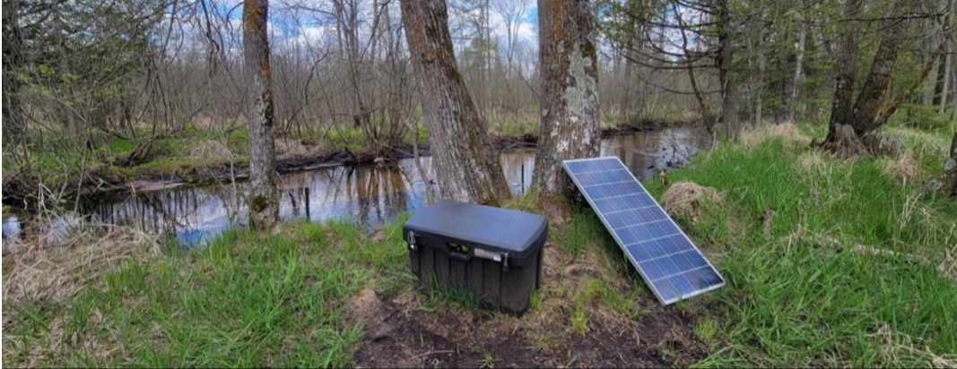
Figure 4: The McMahan PIT array system was installed downstream of the McMahan Road crossing on public land. Image of the McMahan fish monitoring system, taken from the left bank of Upper Middle Inlet. The multi-reader, auto-tuners and deep-cycle marine batteries are located within the black locking box. The 120-watt solar panel is located to the right.
