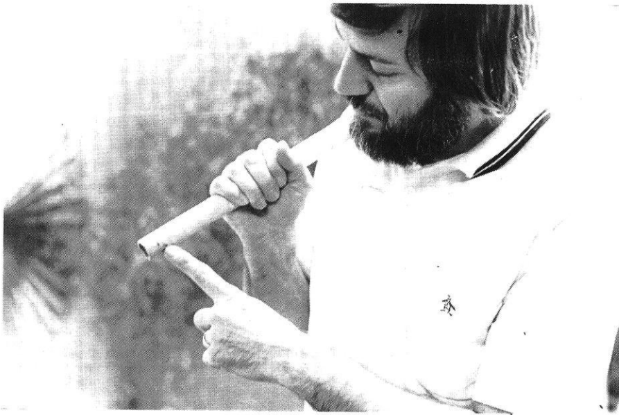
Professor Moll points to missing part of the bottom of an aluminum bat that one of his students investigated. Similar defective bats have caused a number of injuries.
